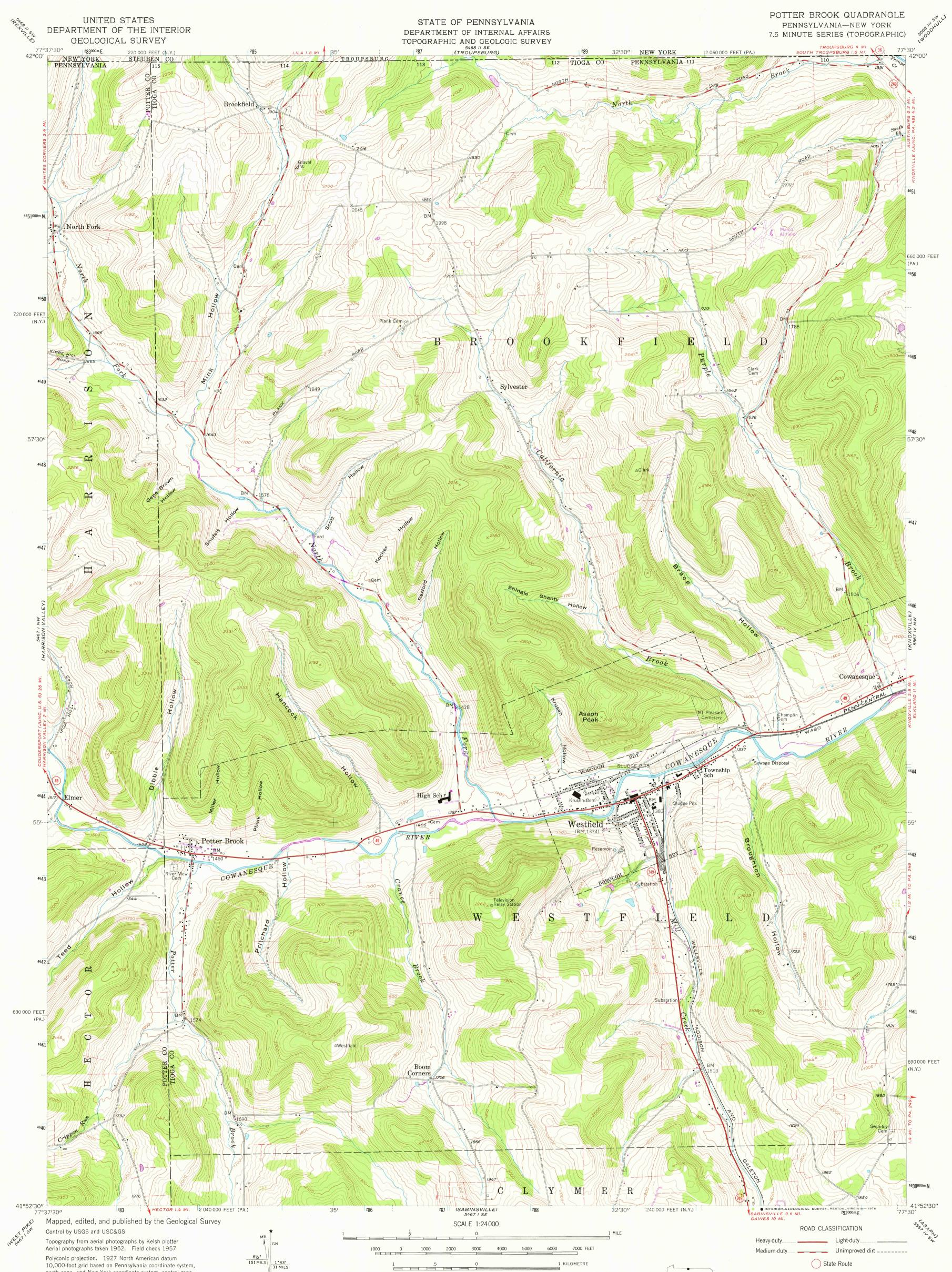
Polyconic projection. 1927 North American datum 10,000-foot grid based on Pennsylvania coordinate system, north zone, and New York coordinate system, central zone 1000-metre Universal Transverse Mercator grid ticks, zone 18, shown in blue
