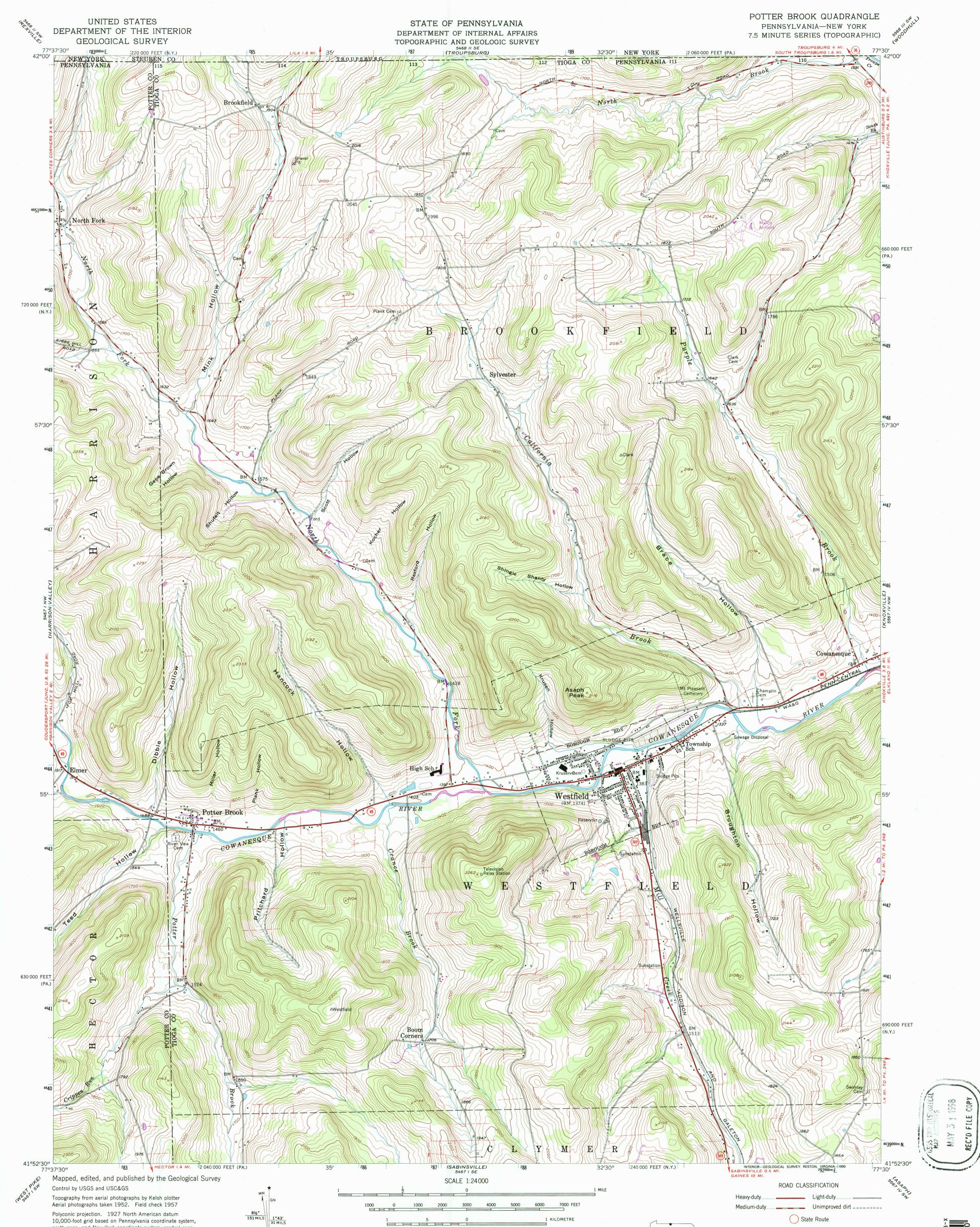
Polyconic projection. 1927 North American datum 10,000-foot grid based on Pennsylvania coordinate system, north zone, and New York coordinate system, central zone 1000-metre Universal Transverse Mercator grid ticks, zone 18, shown in blue
