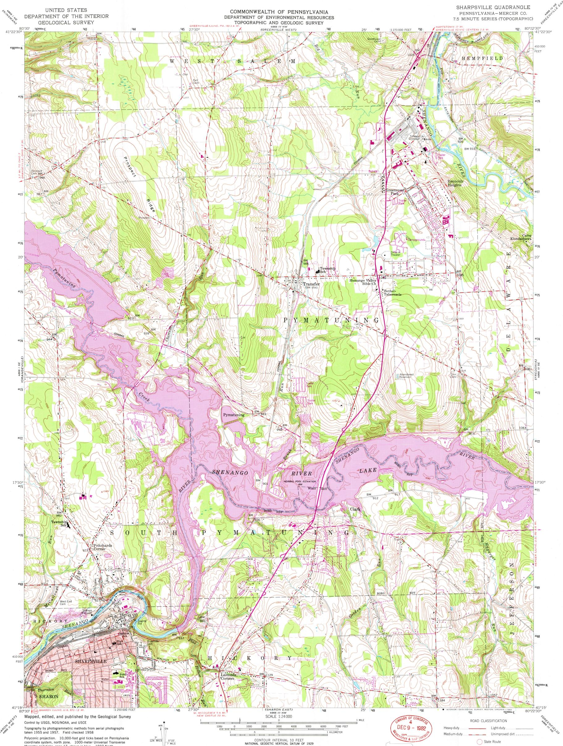
Polyconic projection. 10,000-foot grid ticks based on Pennsylvania coordinate system, north zone. 1000-meter Universal Transverse Mercator grid ticks, zone 17, shown in blue. 1927 North American Datum. To place on the predicted North American Datum 1983 move the projection lines 2 meters south and 17 meters west as shown by dashed corner ticks
