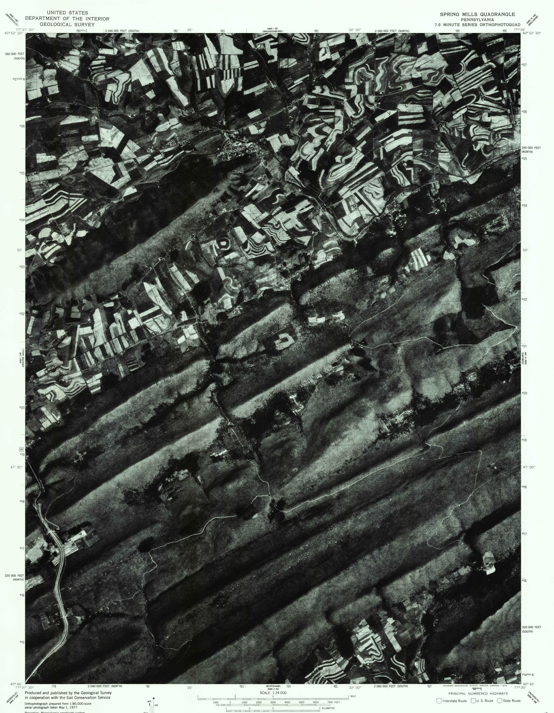
Projection: Pennsylvania coordinate system, north zone (Lambert conformal conic) 10,000-foot grid ticks based on Pennsylvania coordinate system, north and south zones 1000-meter Universal Transverse Mercator grid ticks, zone 18. 1927 North American datum Photoimagery rectified by automatic correlation
