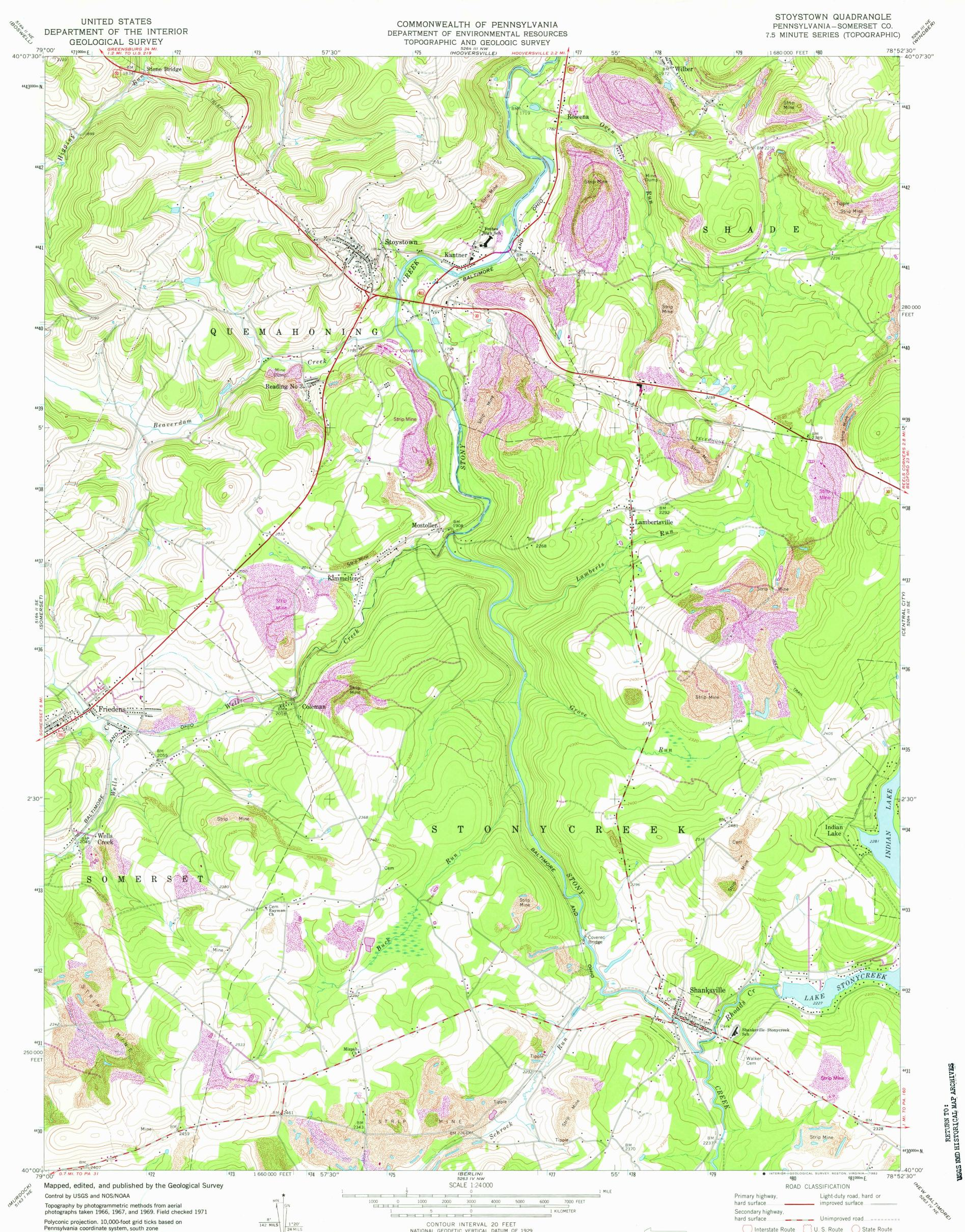
Polyconic projection. 10,000-foot grid ticks based on Pennsylvania coordinate system, south zone 1000-meter Universal Transverse Mercator grid ticks, zone 17, shown in blue. 1927 North American Datum To place on the predicted North American Datum 1983 move the projection lines 5 meters south and 21 meters west as shown by dashed corner ticks
