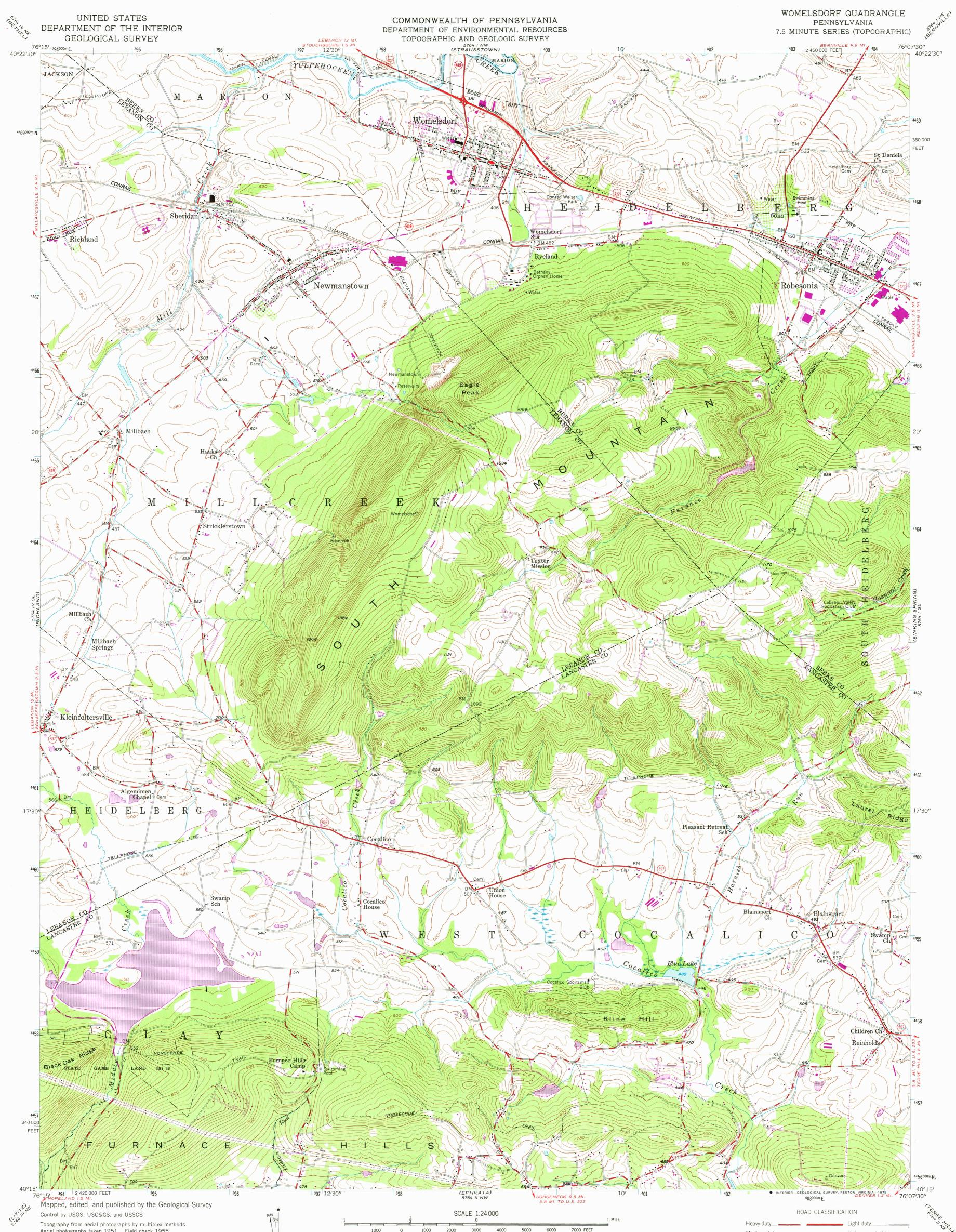
Aerial photographs taken 1951. Field check 1955 Polyconic projection. 1927 North American datum 10,000-foot grid based on Pennsylvania coordinate system, south zone 1000-meter Universal Transverse Mercator grid ticks, zone 18, shown in blue UTM GRID AND 1977 MAGNETIC NORTH DECLINATION AT CENTER OF SHEET Revisions shown in purple compiled in cooperation with State of Pennsylvania agencies from aerial photographs taken 1969 and 1976 This information not field checked. Map edited 1977
