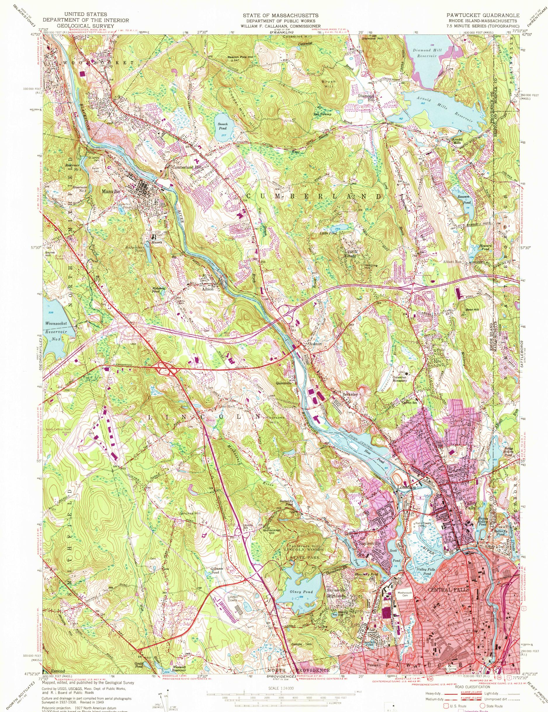
Polyconic projection. 1927 North American datum 10,000-foot grids based on Rhode Island coordinate system and Massachusetts coordinate system (Mainland)
