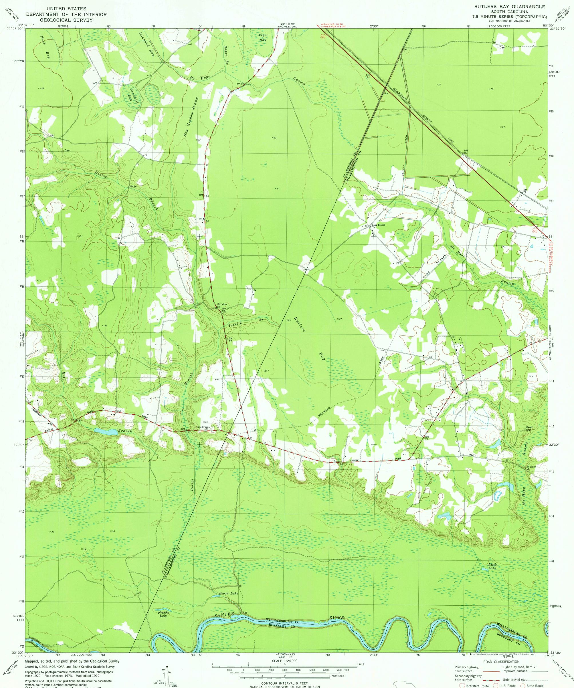
system, south zone (Lambert conformal conic) 1000-meter Universal Transverse Mercator grid, zone 17 1927 North American Datum To place on the predicted North American Datum 1983 move the projection lines 14 meters south and 19 meters west as shown by dashed corner ticks
