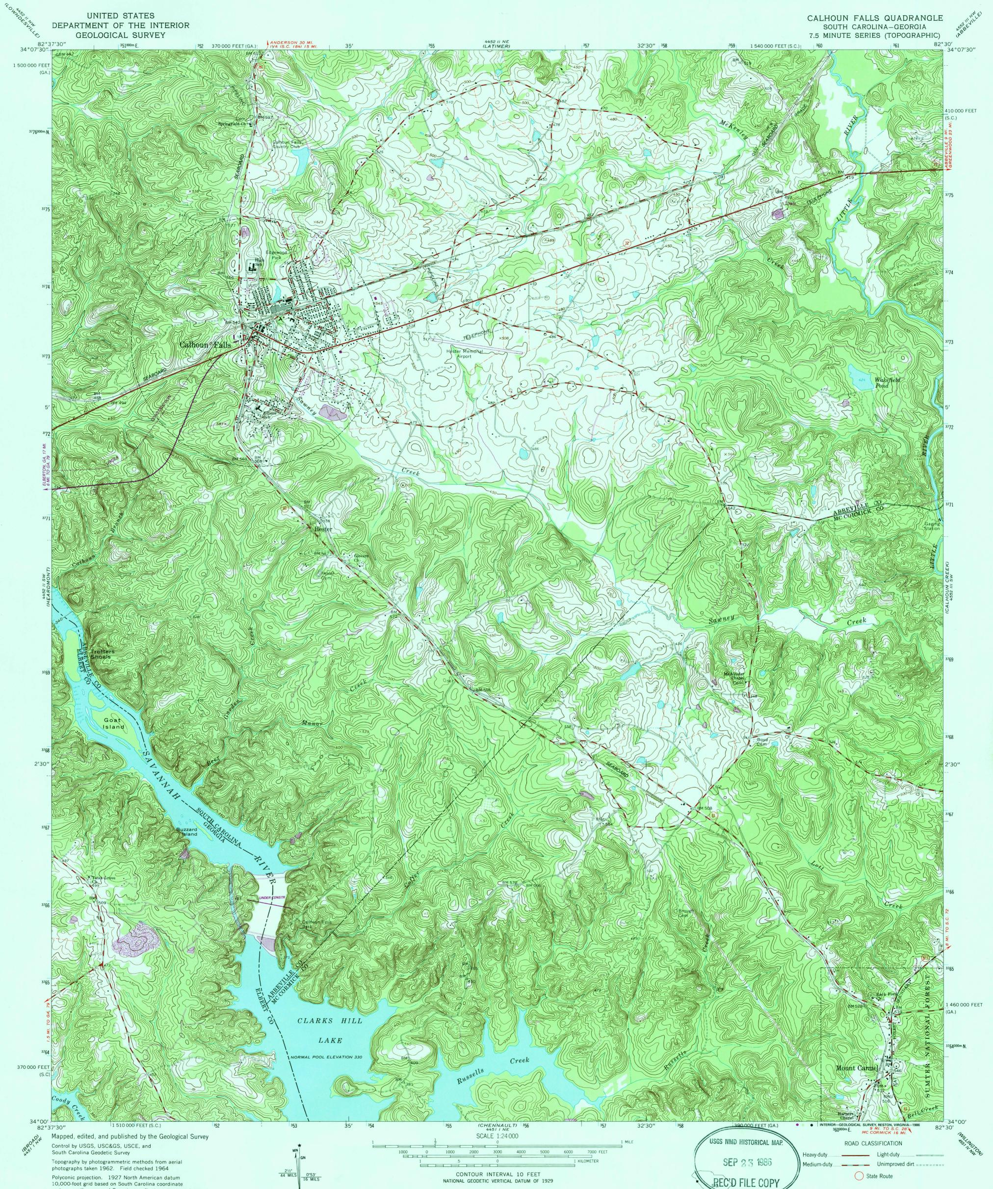
Polyconic projection. 1927 North American datum 10,000-foot grid based on South Carolina coordinate system, north zone, and Georgia coordinate system, east zone 1000-meter Universal Transverse Mercator grid ticks, zone 17, shown in blue To place on the predicted North American Datum 1983, move the projection lines 11 meters south and 13 meters west as shown by dashed corner ticks
