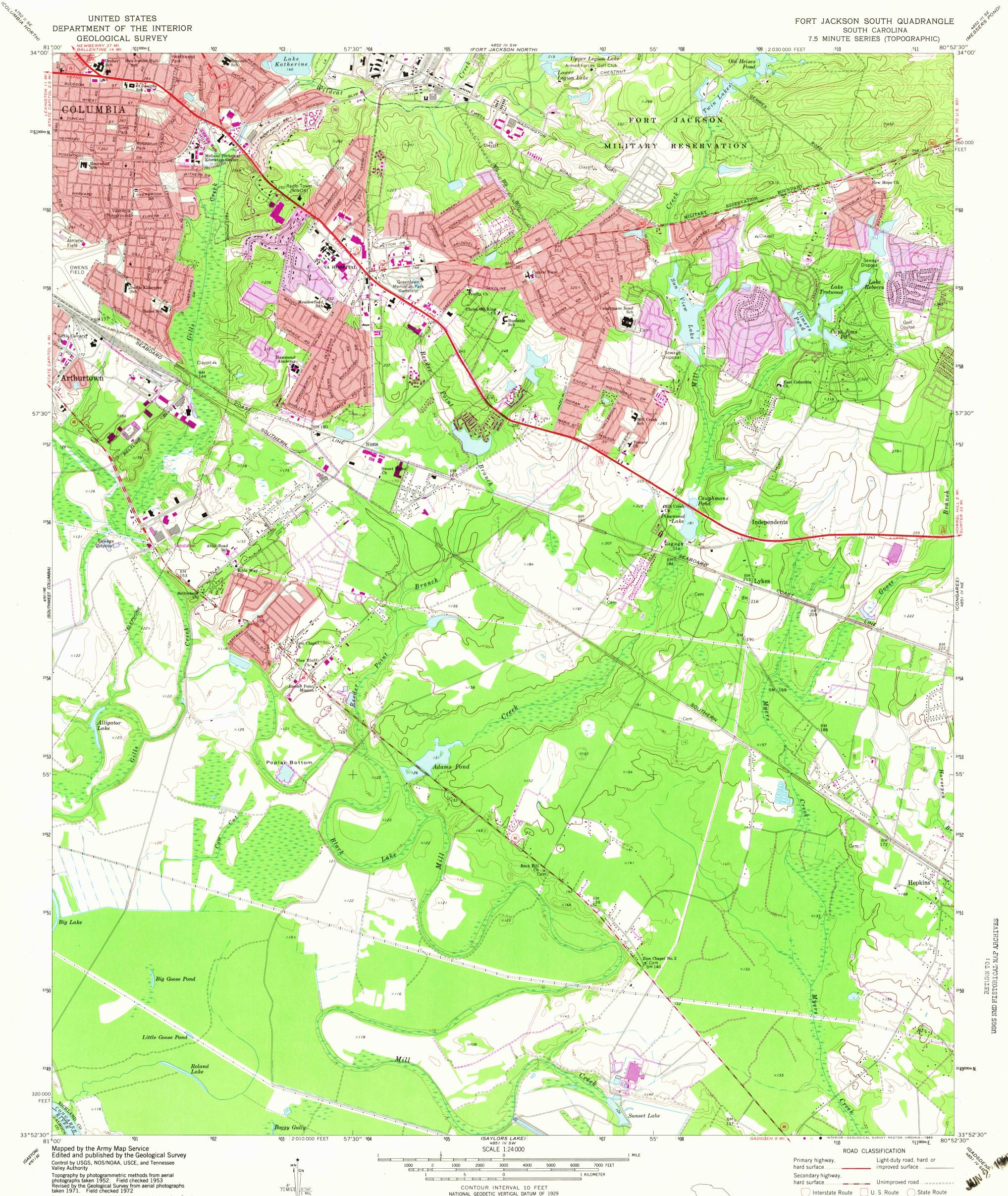
Polyconic projection. 10,000-foot grid ticks based on South Carolina coordinate system, north zone. 1000-meter Universal Transverse Mercator grid ticks, zone 17, shown in blue. 1927 North American Datum To place on the predicted North American Datum 1983 move the projection lines 12 meters south and 17 meters west as shown by dashed corner ticks
