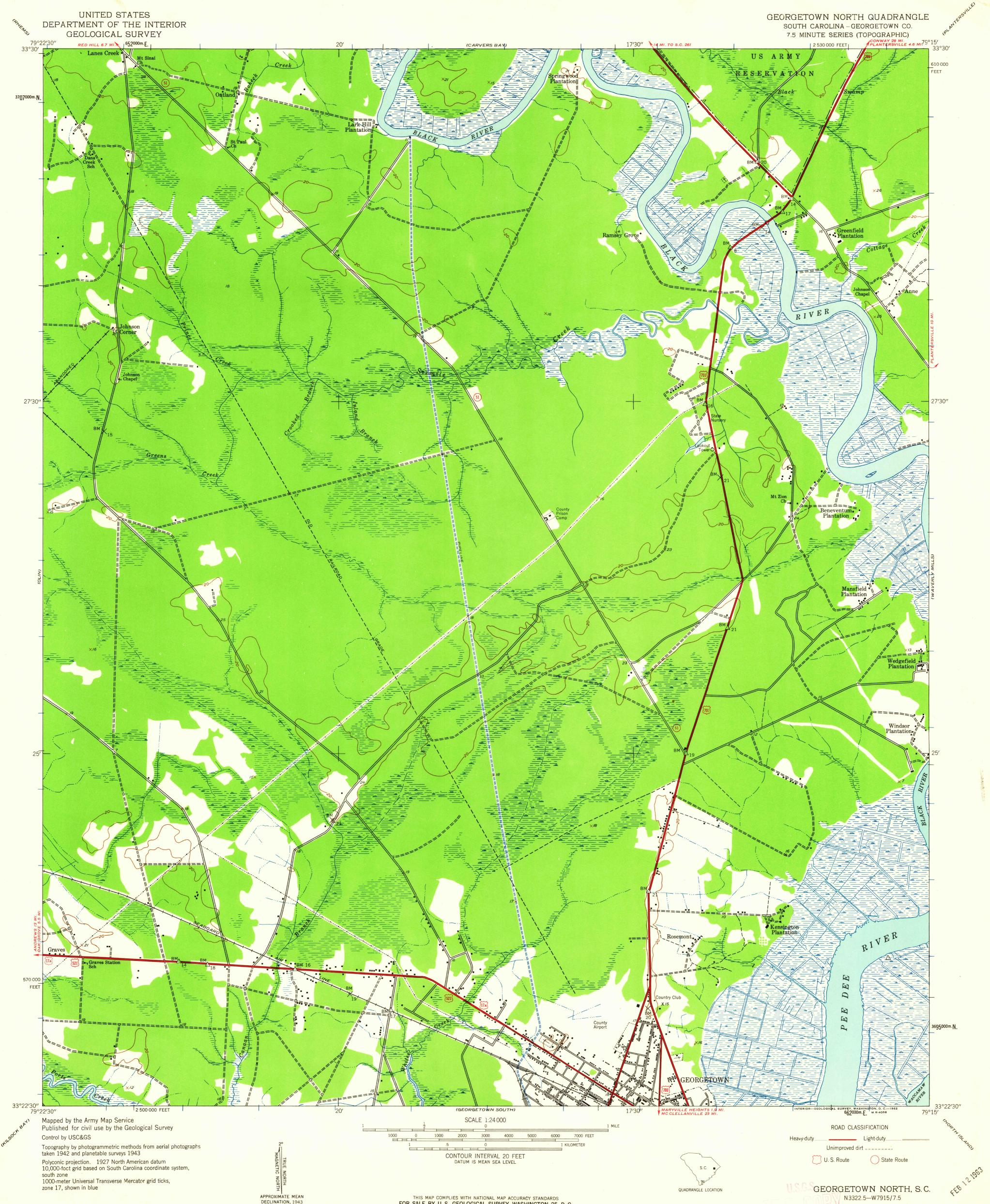
Polyconic projection. 1927 North American datum 10,000-foct grid based on South Carolina coordinate system, south zone 1000-meter Universal Transverse Mercator grid ticks, zone 17, shown in blue
