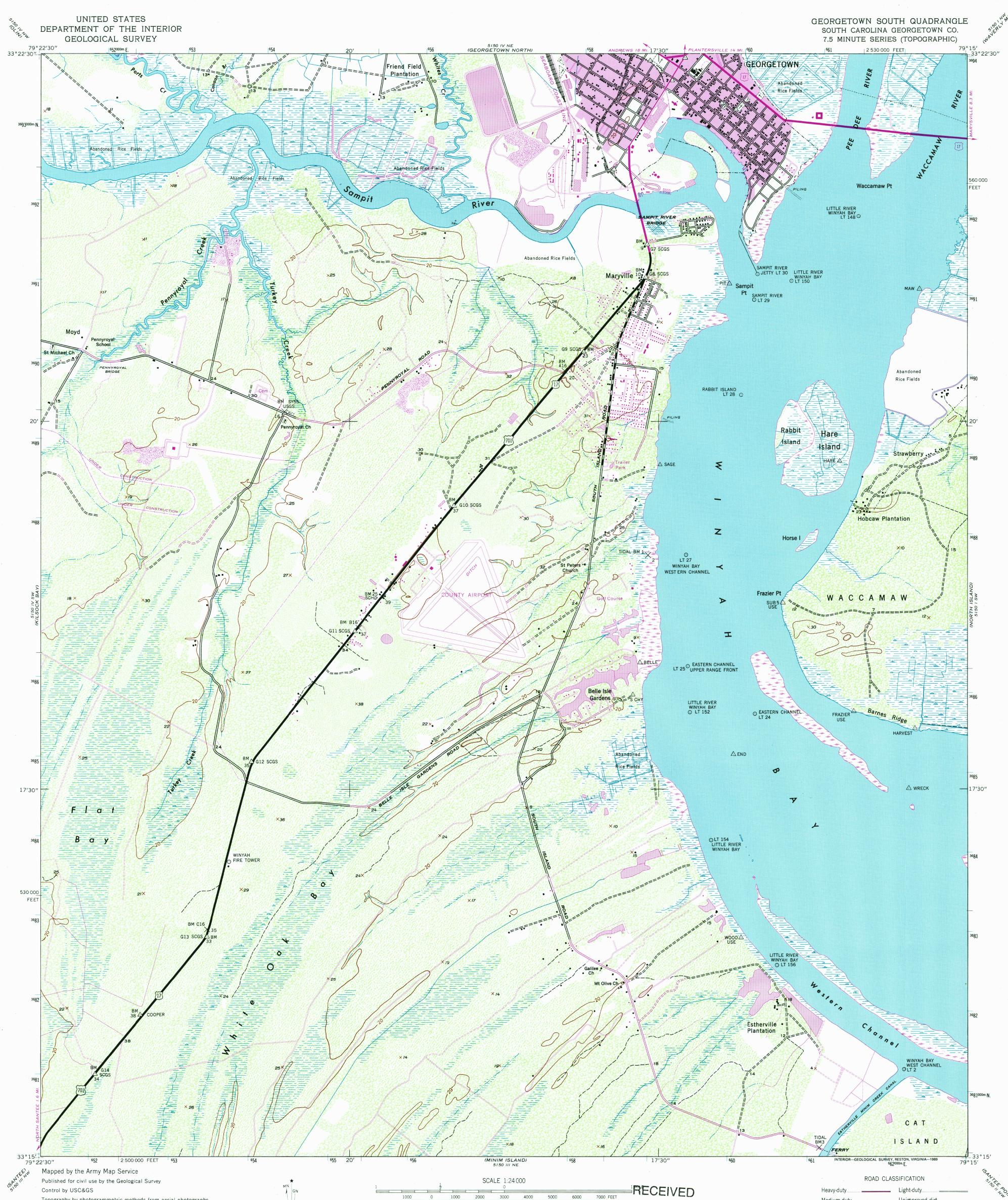
Topography by photogrammetric methods from aerial photographs taken 1942 and planetable surveys 1943 Transverse Mercator projection. 1927 North American datum 10,000-foot grid based on South Carolina coordinate system, south zone
