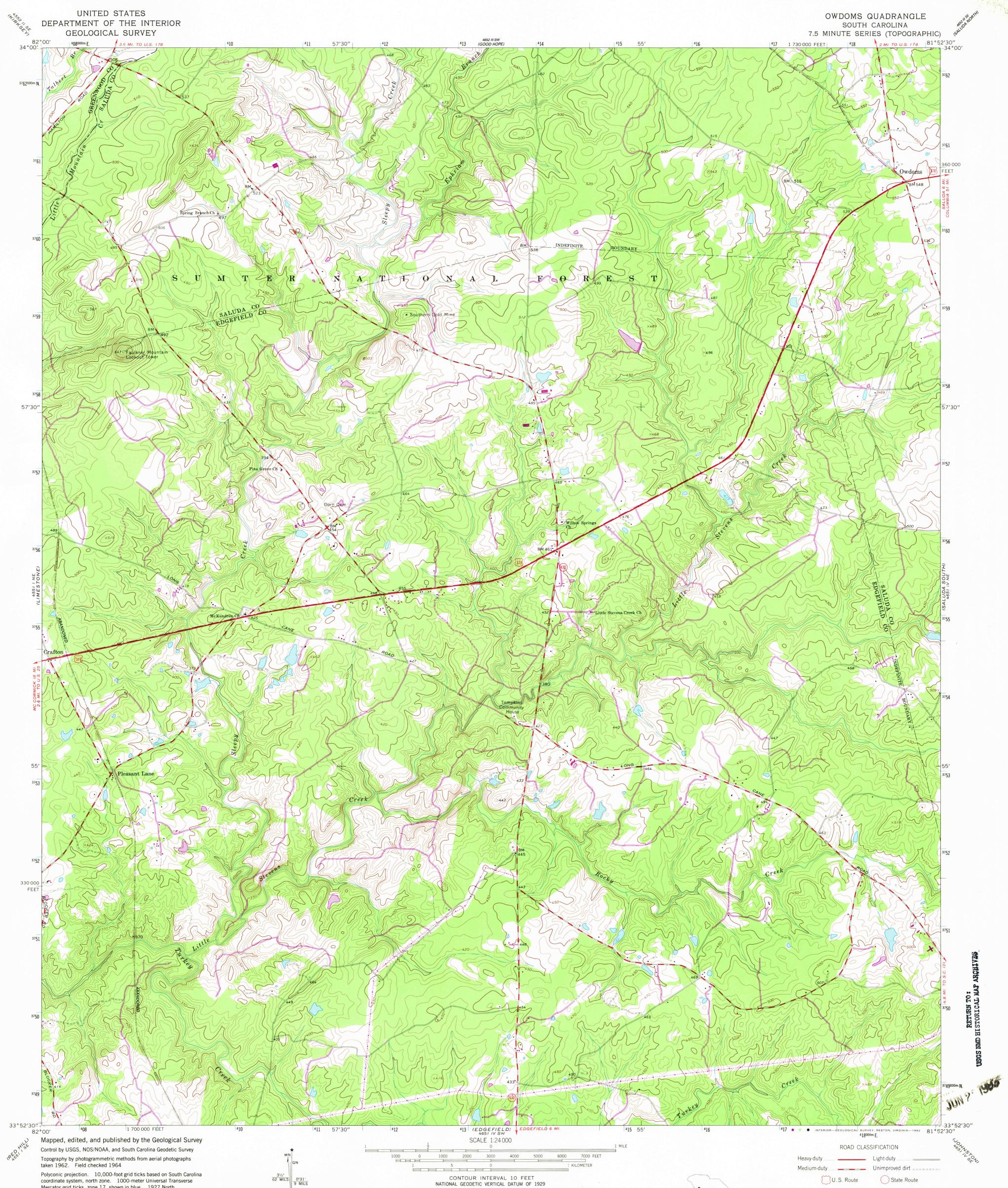
coordinate system, north zone. 1000-meter Universal Transverse Mercator grid ticks, zone 17, shown in blue. 1927 North American Datum. To place on the predicted North American Datum 1983 move the projection lines 12 meters south and 15 meters west as shown by dashed corner ticks
