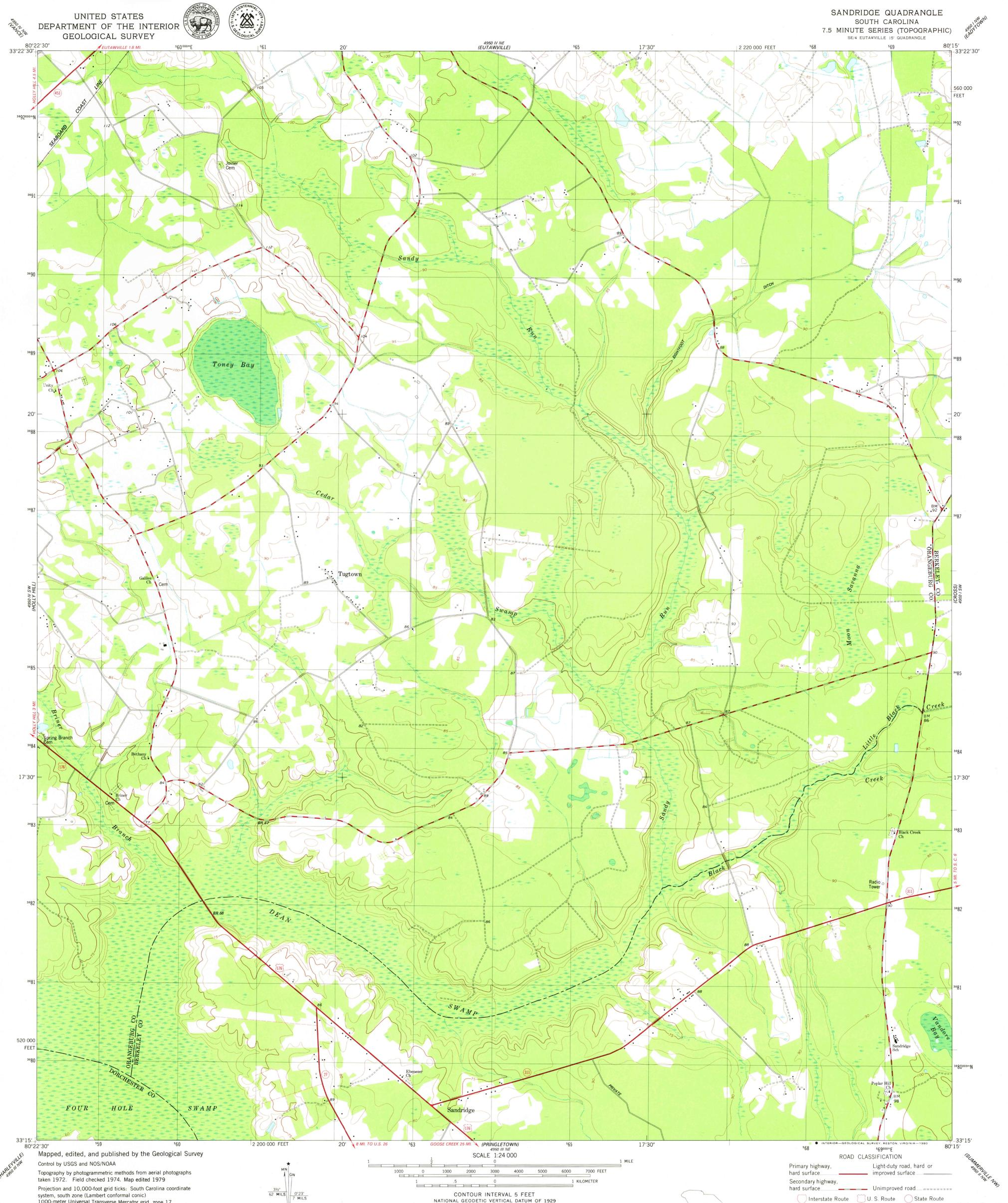
system, south zone (Lambert conformal conic) 1000-meter Universal Transverse Mercator grid, zone 17 1927 North American datum To place on the predicted North American Datum 1983 move the projection lines 14 meters south and 18 meters west as shown by dashed corner ticks
