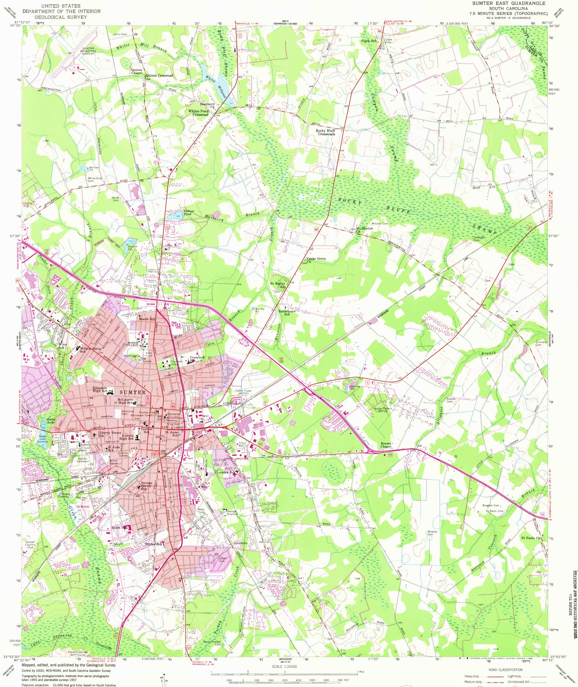
coordinate system, north zone. 1000-meter Universal Transverse Mercator grid ticks, zone 17, shown in blue. 1927 North American Datum. To place on the predicted North American Datum 1983 move the projection lines 13 meters south and 19 meters west as shown by dashed corner ticks
