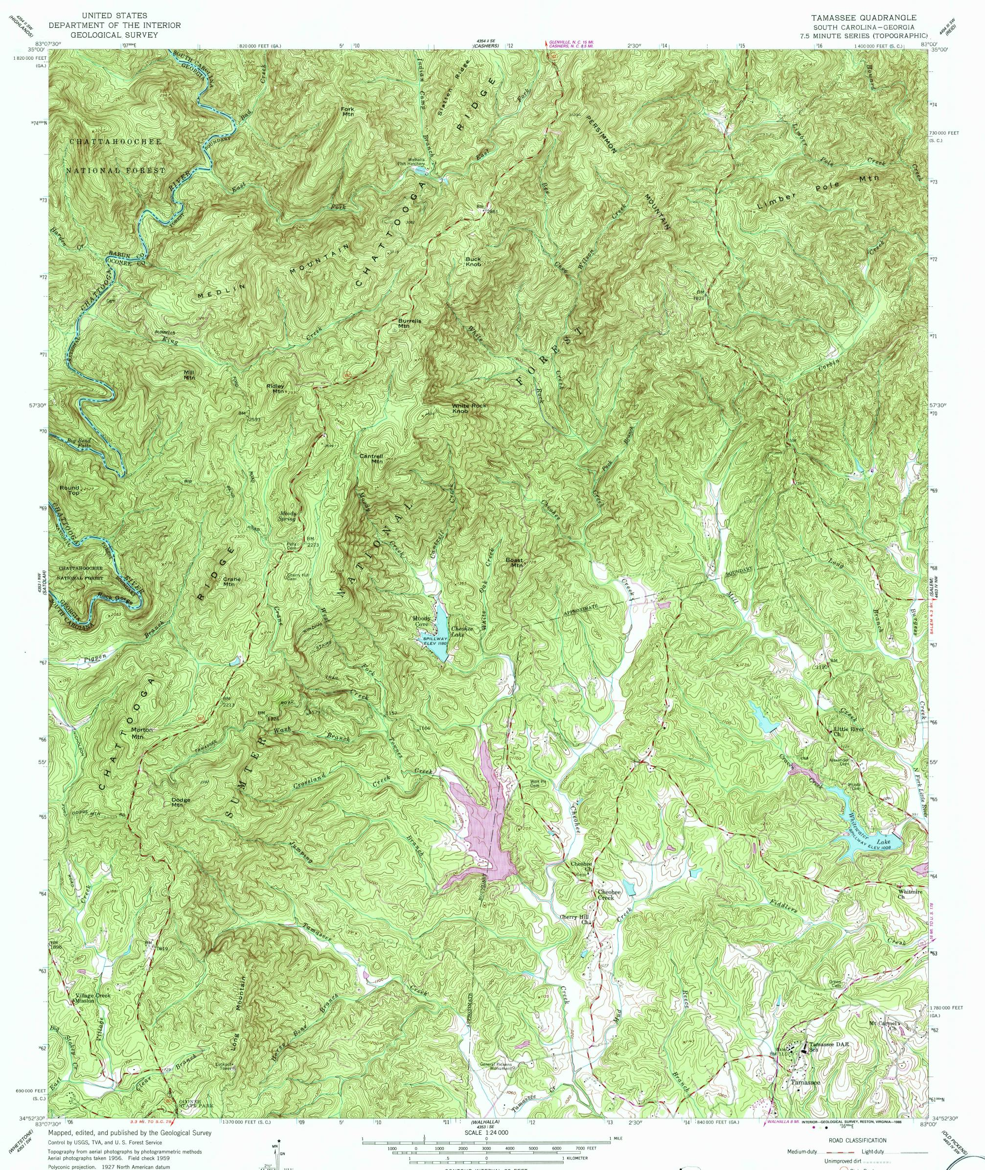
10,000-foot grids based on South Carolina coordinate system, north zone, and Georgia coordinate system, west zone 1000-meter Universal Transverse Mercator grid ticks, zone 17, shown in blue
