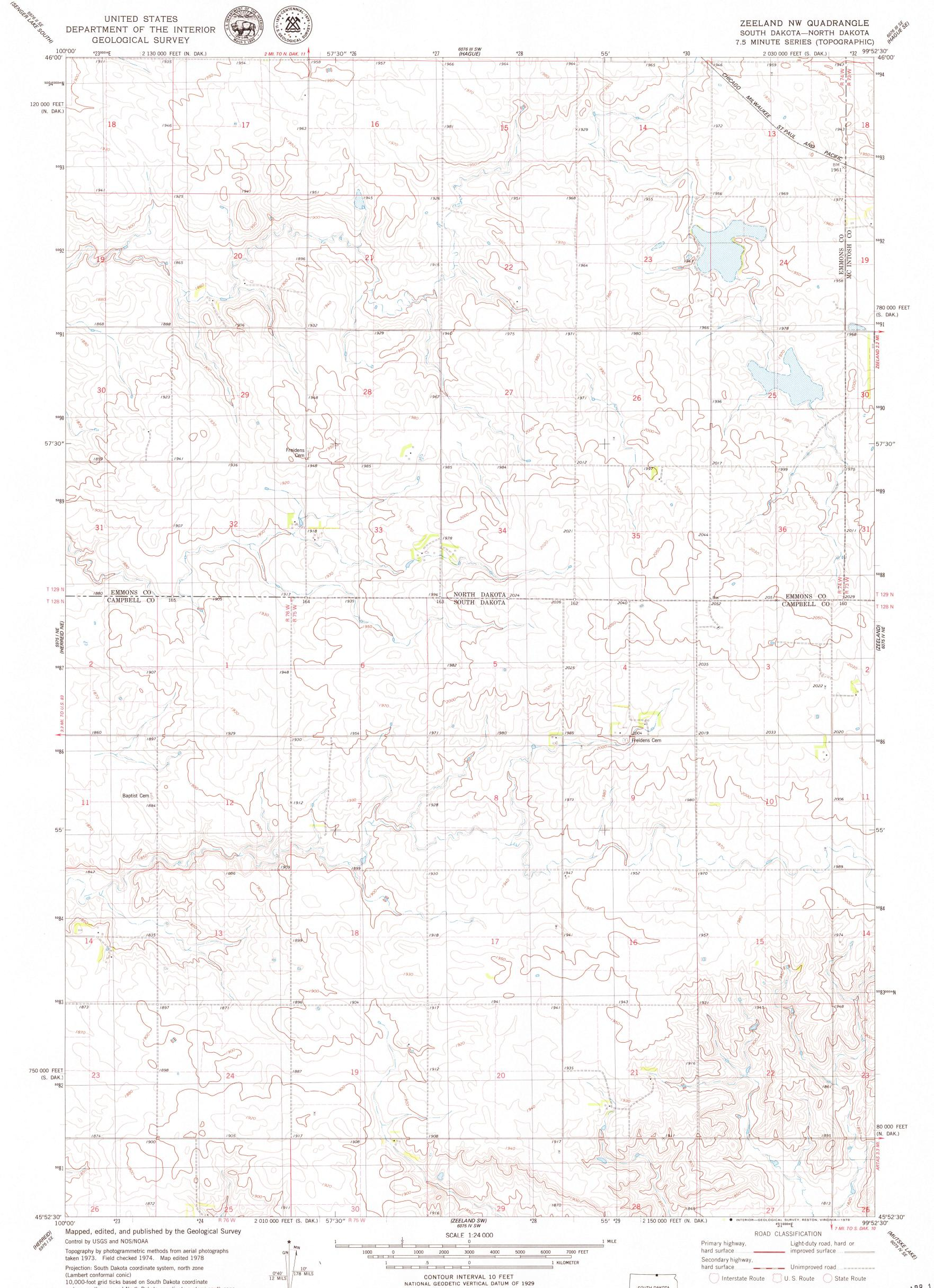
(Lambert conformal conic) 10,000-foot grid ticks based on South Dakota coordinate system, north zone and North Dakota coordinate system, south zone 1000-meter Universal Transverse Mercator grid, zone 14 1927 North American datum Fine red dashed lines indicate selected fence and field lines where generally visible on aerial photographs. This information is unchecked
