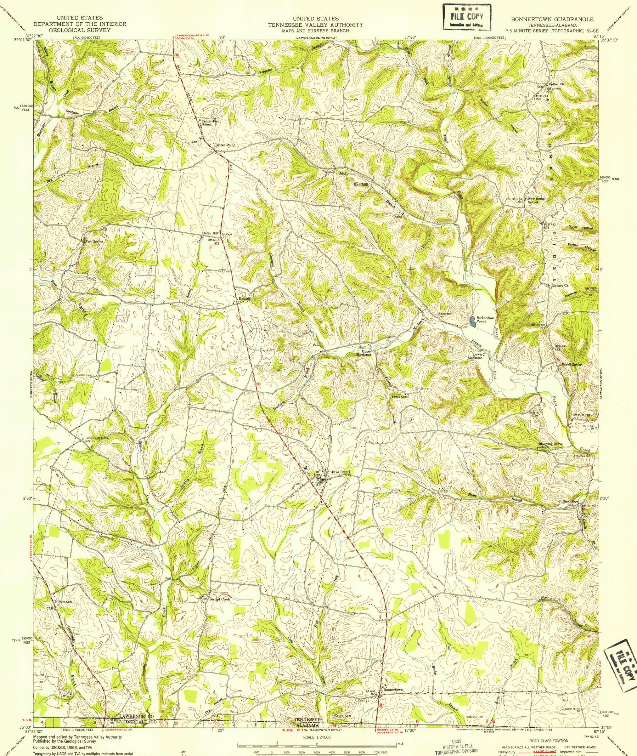
Topography by USGS and TVA by multiplex methods from aerial photographs taken 1946. Field examination by TVA, 1950
