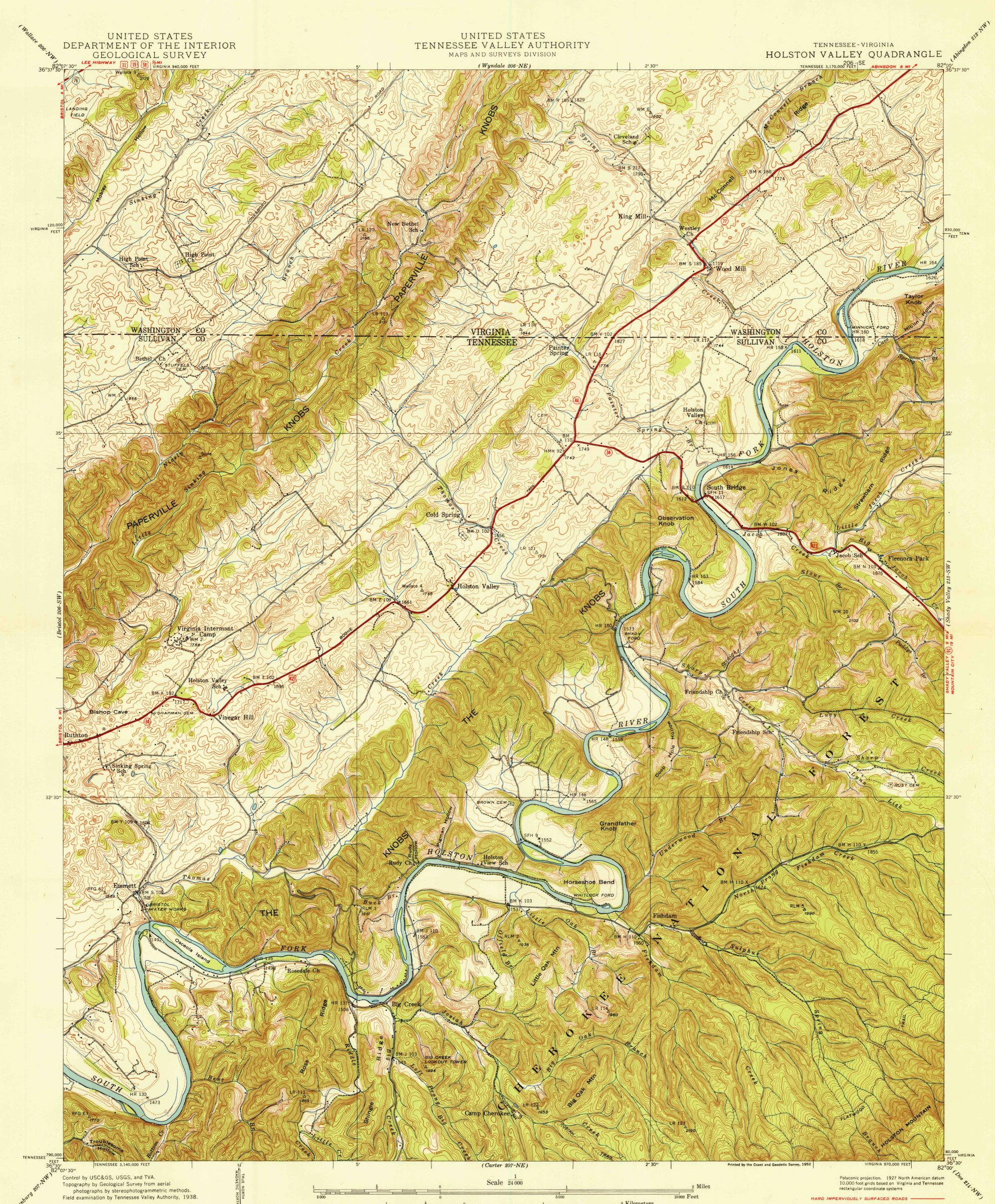
Control by USC&GS, USGS, and TVA. Topography by Geological Survey from aerial photographs by stereophotogrammetric methods. Eield examination by Tennessee Valley Authority, 1938.
