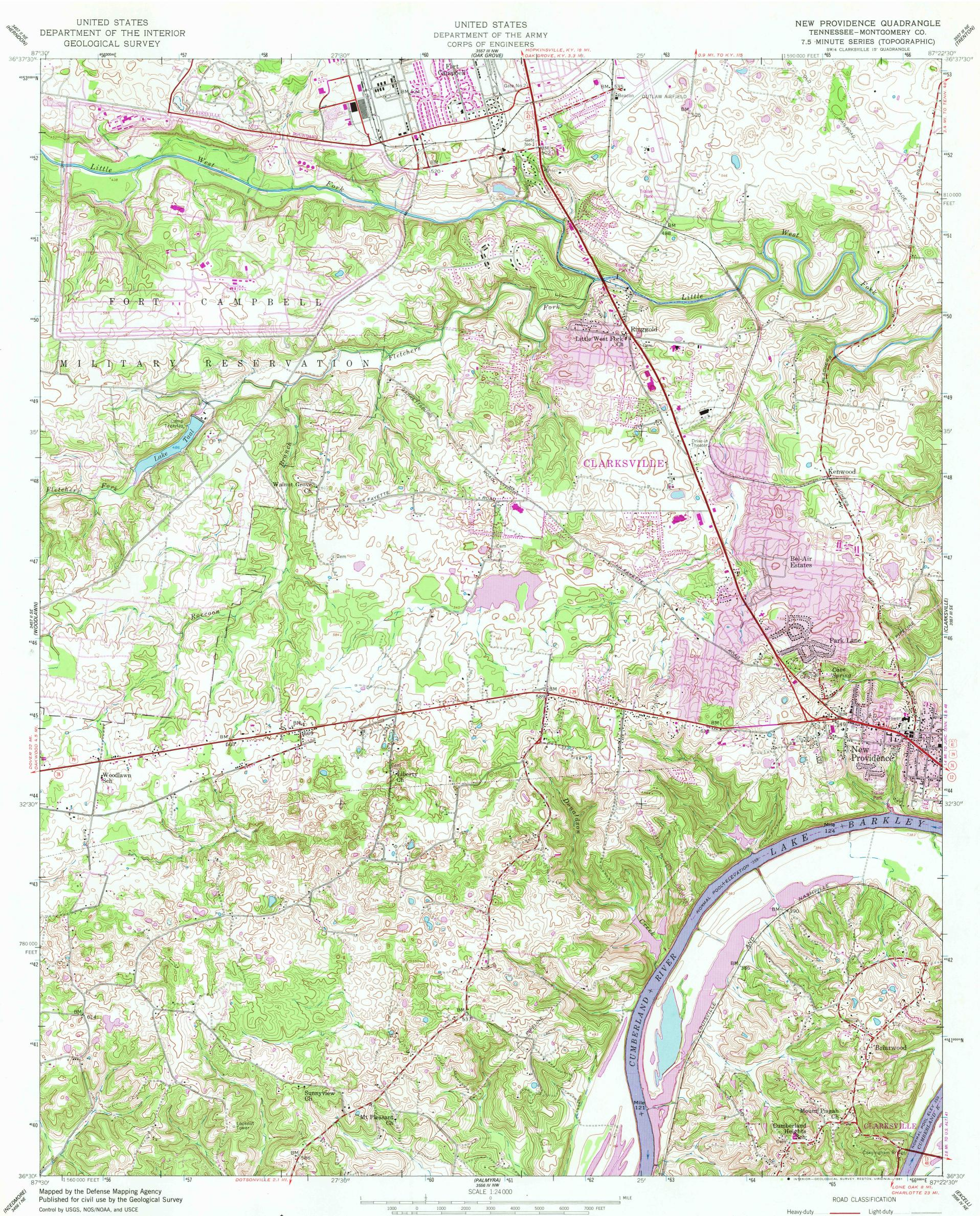
Topography by photogrammetric methods from aerial photographs taken 1951. Planimetric detail revised from aerial photographs taken 1956. Field checked 1957
