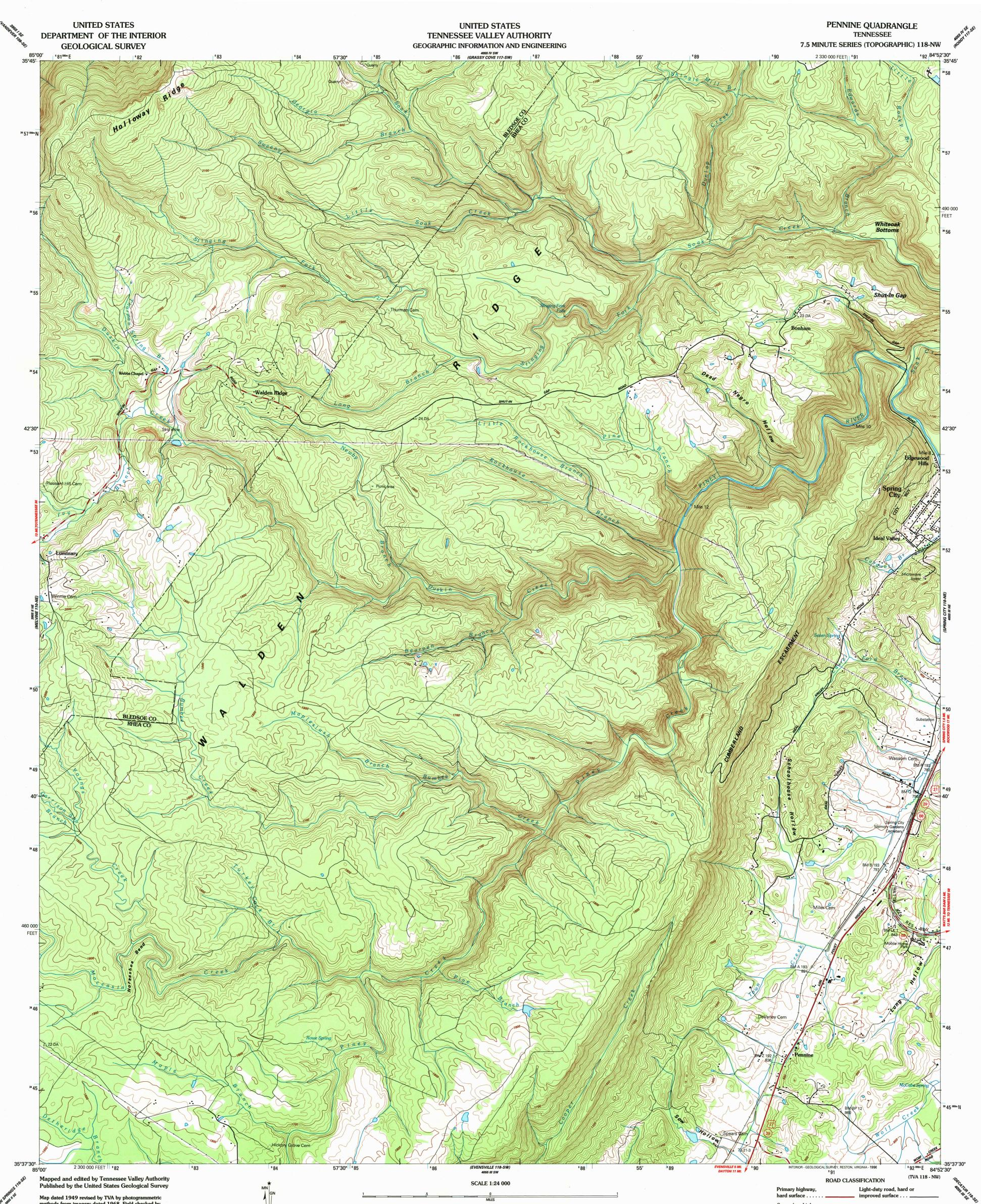
Map dated 1949 revised by TVA by photogrammetric methods from imagery dated 1968. Field checked by TVA 1973. Revised by the U.S. Geological Survey in cooperation with TVA from imagery dated 1990 Survey control current as of 1973 Map edited 1991. Contours not revised
