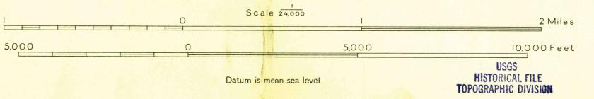
Polyconic projection. 1927 North American datum 10,000 foot grid based on Tennessee rectangular coordinate system
