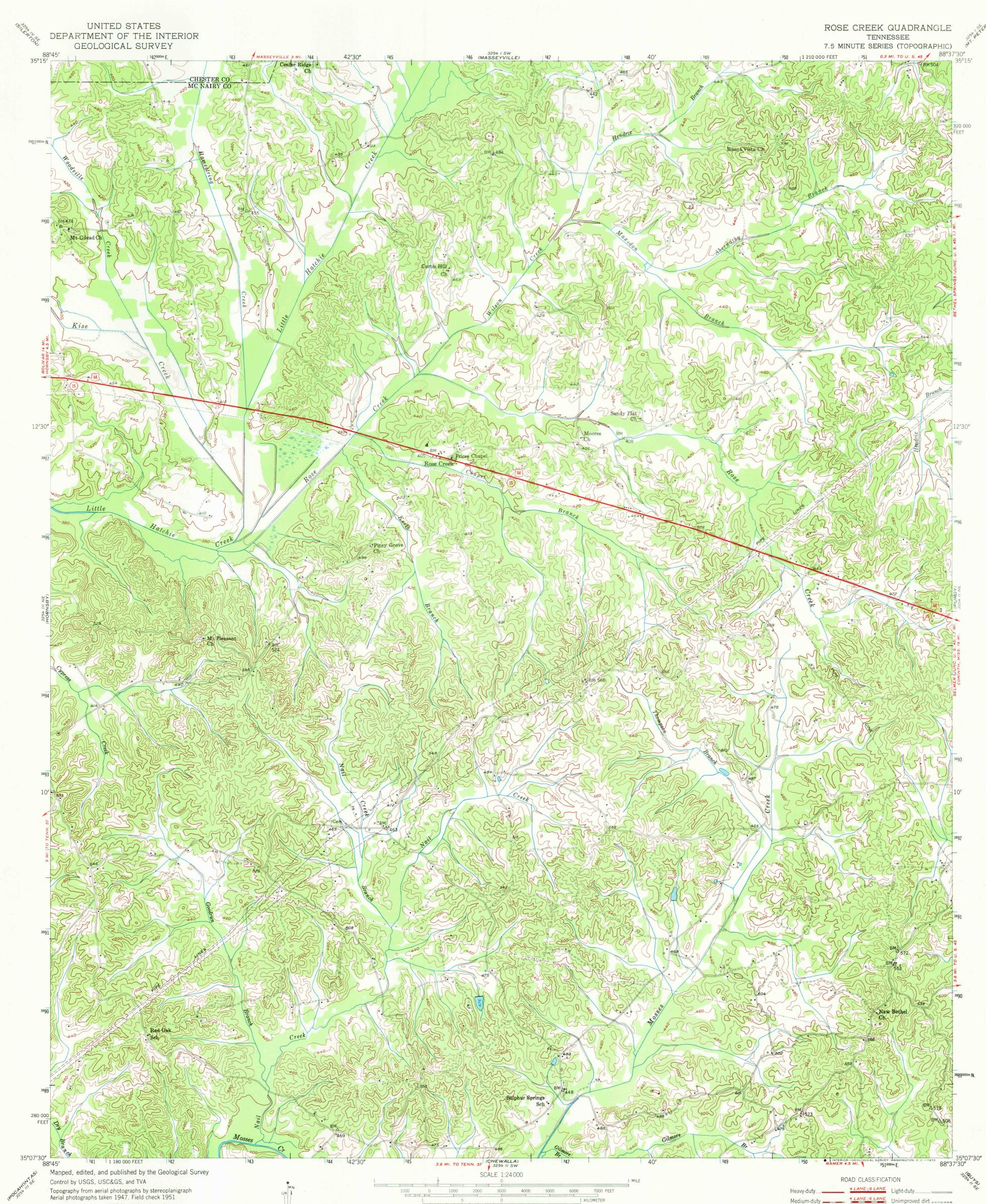
Topography from aerial photographs by stereoplanigraph Aerial photographs taken 1947. Field check 1951 Polyconic projection. 1927 North American datum 10,000-foot grid based on Tennessee coordinate system 1000-meter Universal Transverse Mercator grid ticks, zone 16, shown in blue
