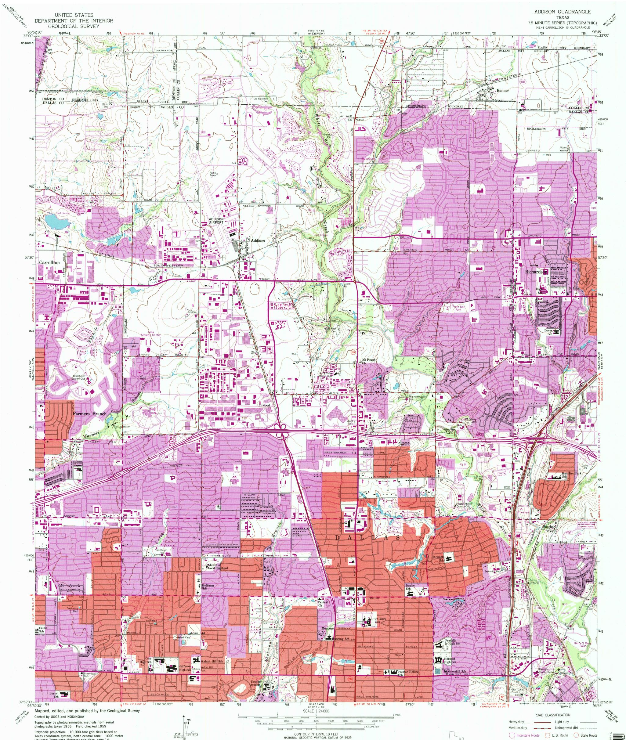
Polyconic projection. 10,000-foot grid ticks based on Texas coordinate system, north central zone. 1000-meter Universal Transverse Mercator grid ticks, zone 14, shown in blue. 1927 North American Datum. To place on the predicted North American Datum 1983 move the projection lines 10 meters south and 26 meters east as shown by dashed corner ticks
