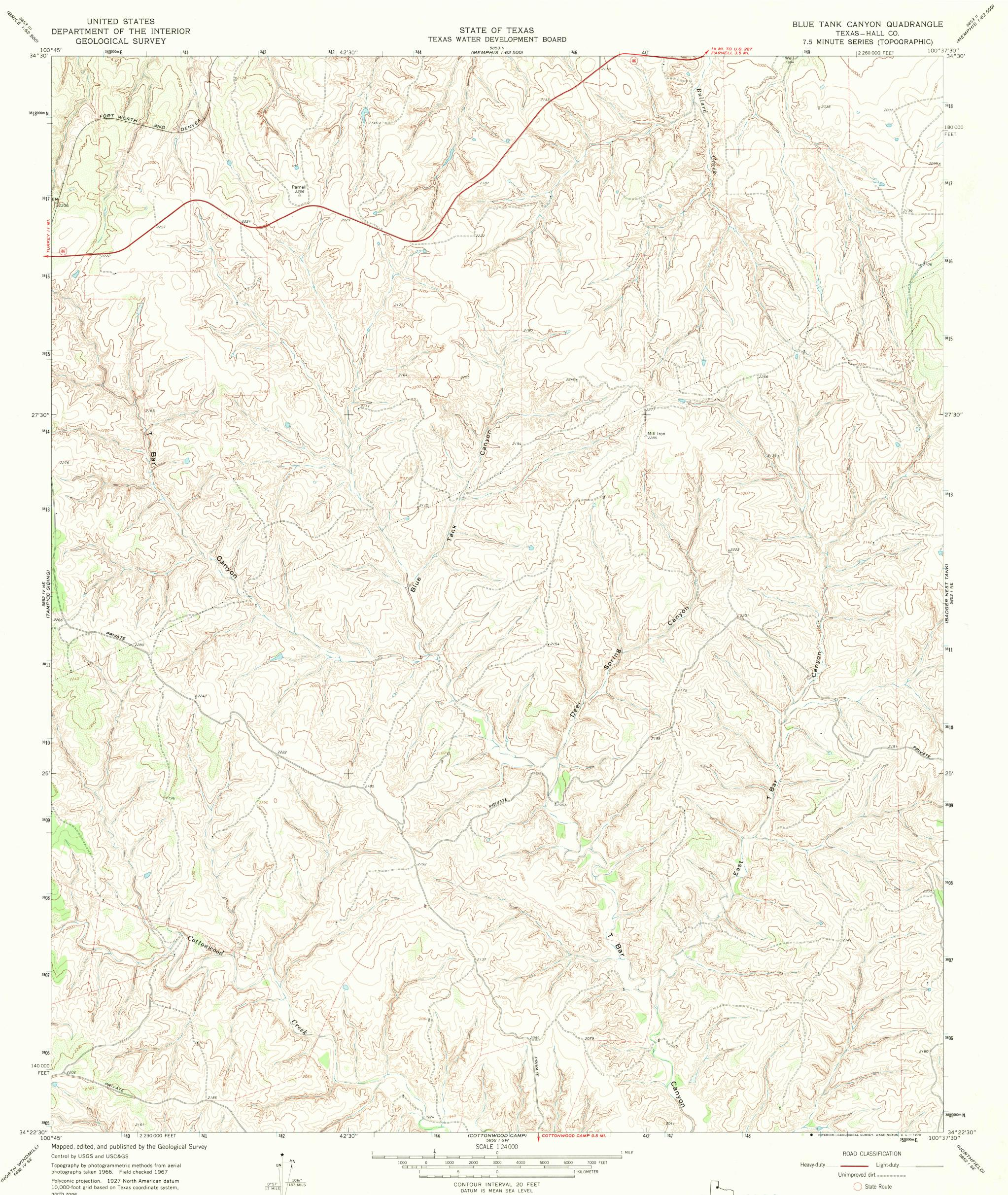
Polyconic projection. 1927 North American datum 10,000-foot grid based on Texas coordinate system, north zone 1000-meter Universal Transverse Mercator grid ticks, zone 14, shown in blue
