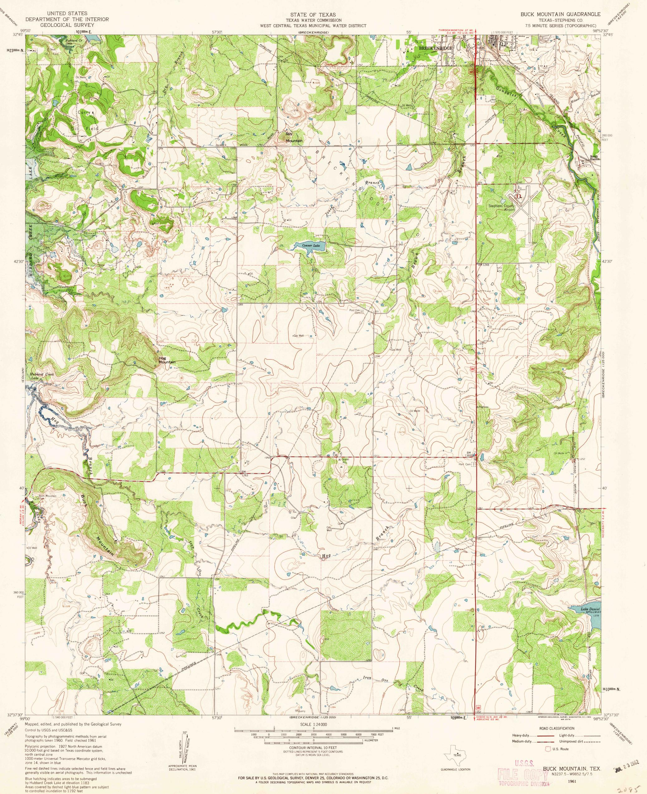
Blue hatching indicates areas to be submerged by Hubbard Creek Lake at elevation 1183 Areas covered by dashed light-blue pattern are subject to controlled inundation to 1192 feet
