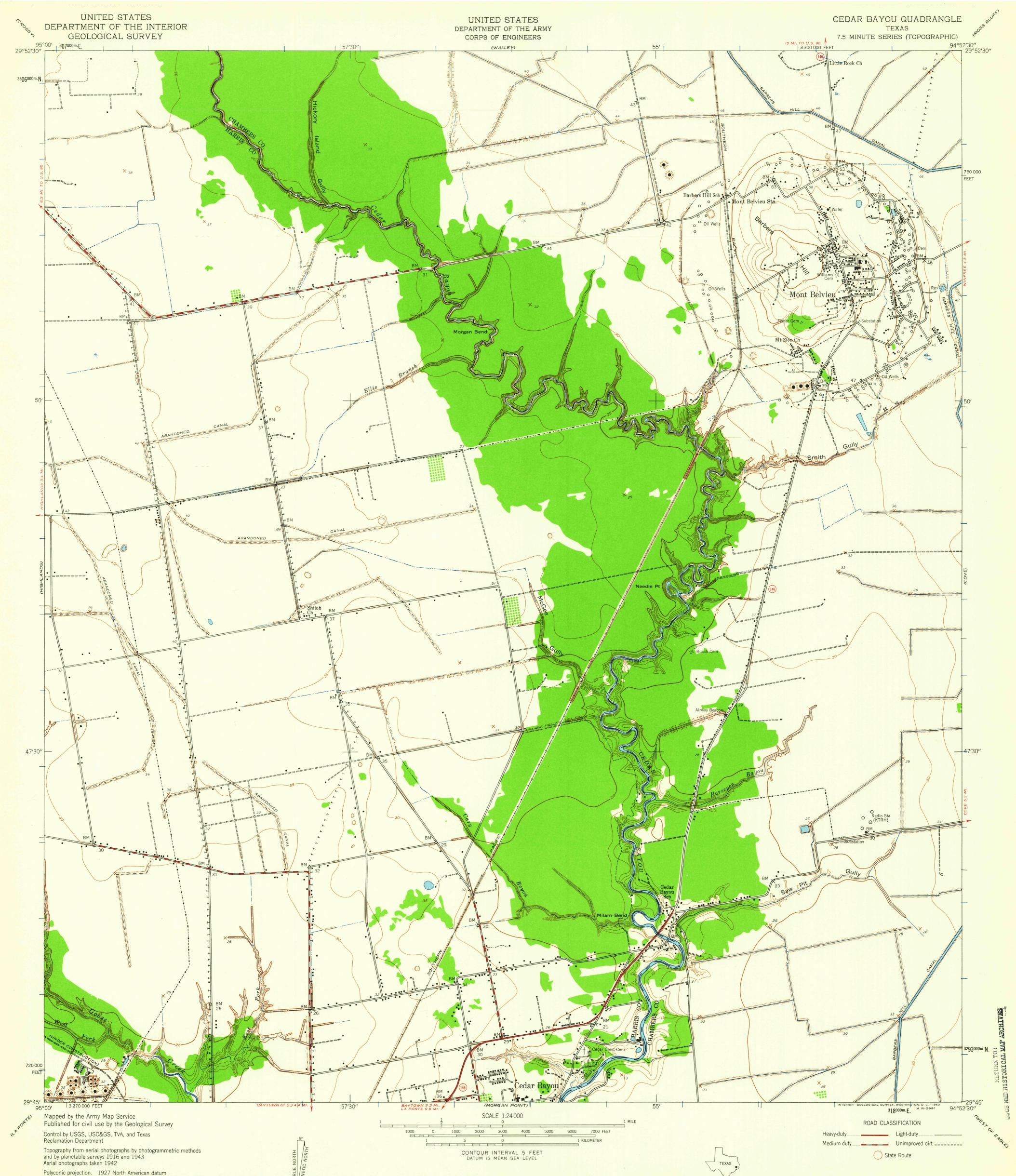
Topography from aerial photographs by photogrammetric methods and by planetable surveys 1916 and 1943 Aerial photographs taken 1942 Polyconic projection. 1927 North American datum 10,000-foot grid based on Texas coordinate system, south central zone 1000-ineter Universal Transverse Mercator grid ticks, zone 15, shown in blue
