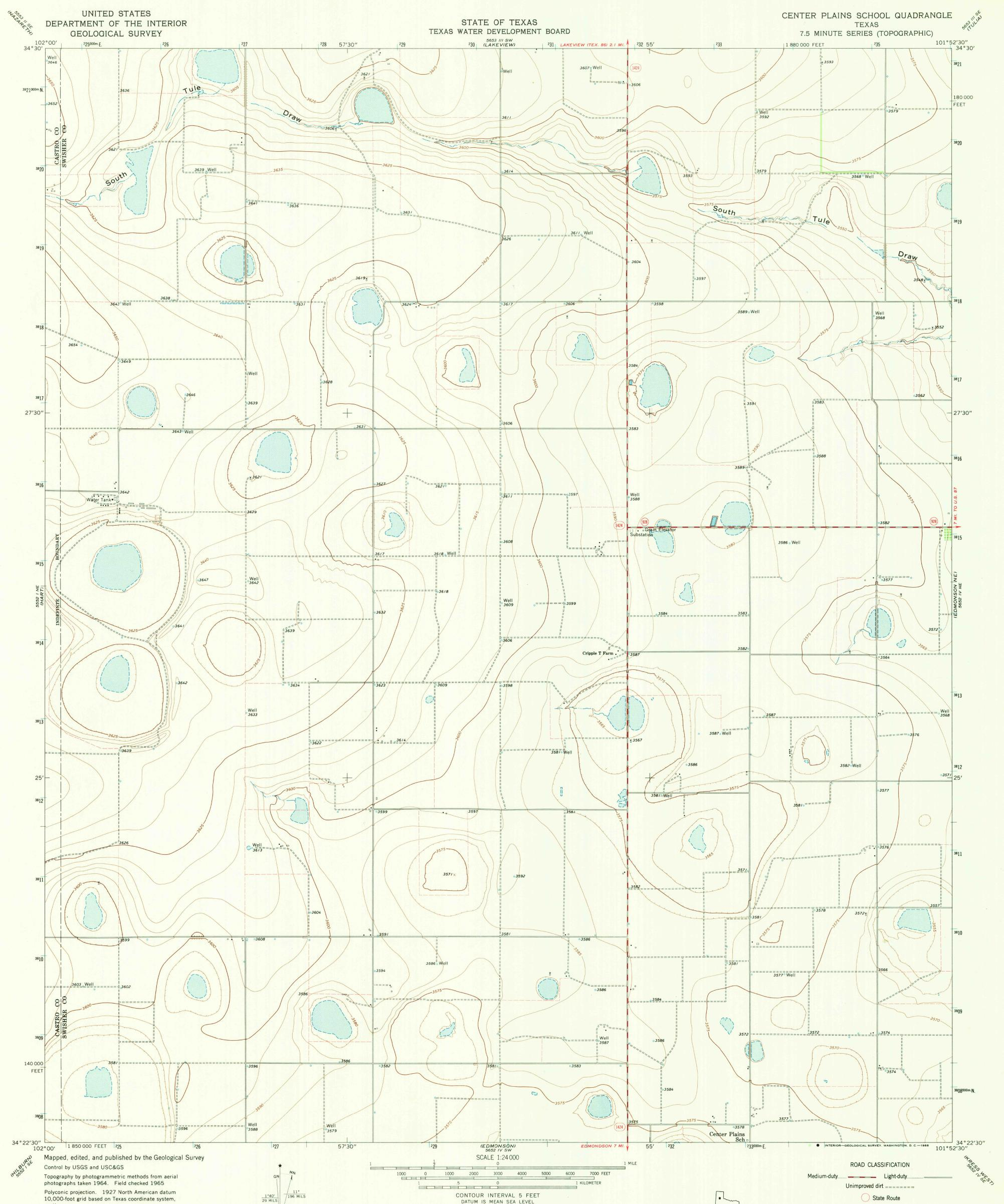
Polyconic projection. 1927 North American datum 10,000-foot grid based on Texas coordinate system, north zone 1000-meter Universal Transverse Mercator grid ticks, zone 14, shown in blue
