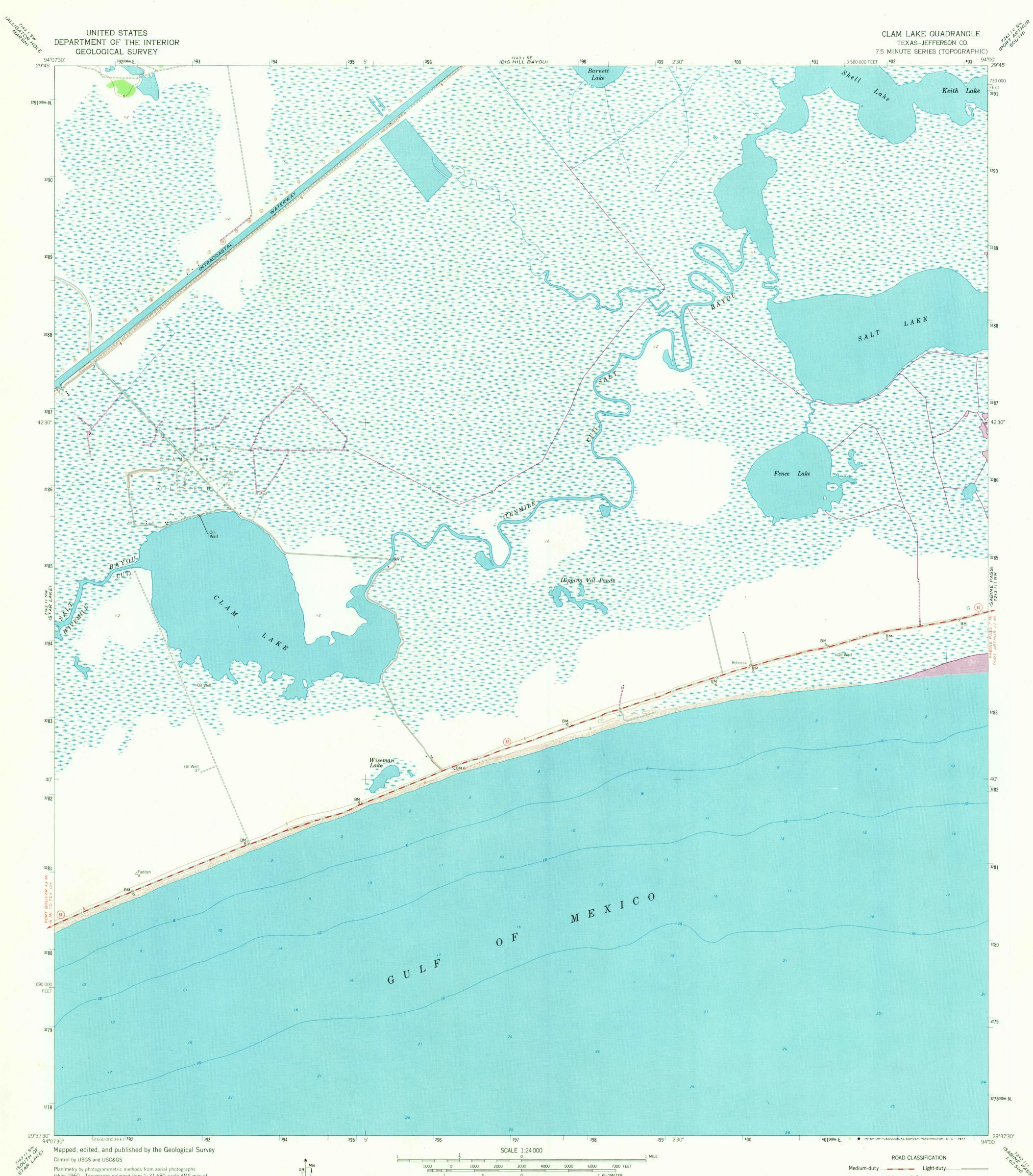
Planimetry by photogrammetric methods from aerial photographs taken 1960. Topography enlarged from 1:31 680-scale AMS map of Clam Lake quadrangle. Original map by photogrammetric methods and planetable surveys 1943. Revised 1961
