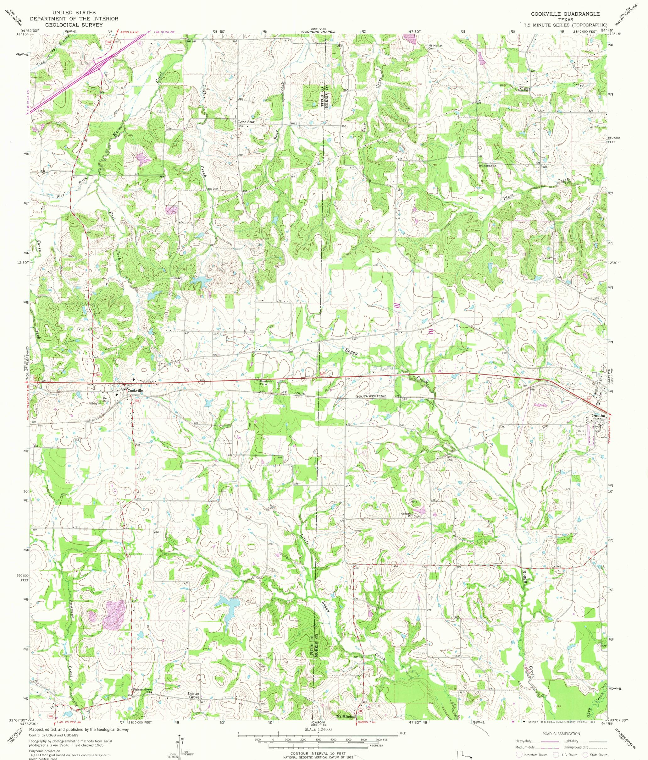
Polyconic projection 10,000-foot grid based on Texas coordinate system, north central zone 1000-meter Universal Transverse Mercator grid ticks, zone 15, shown in blue. 1927 North American Datum
