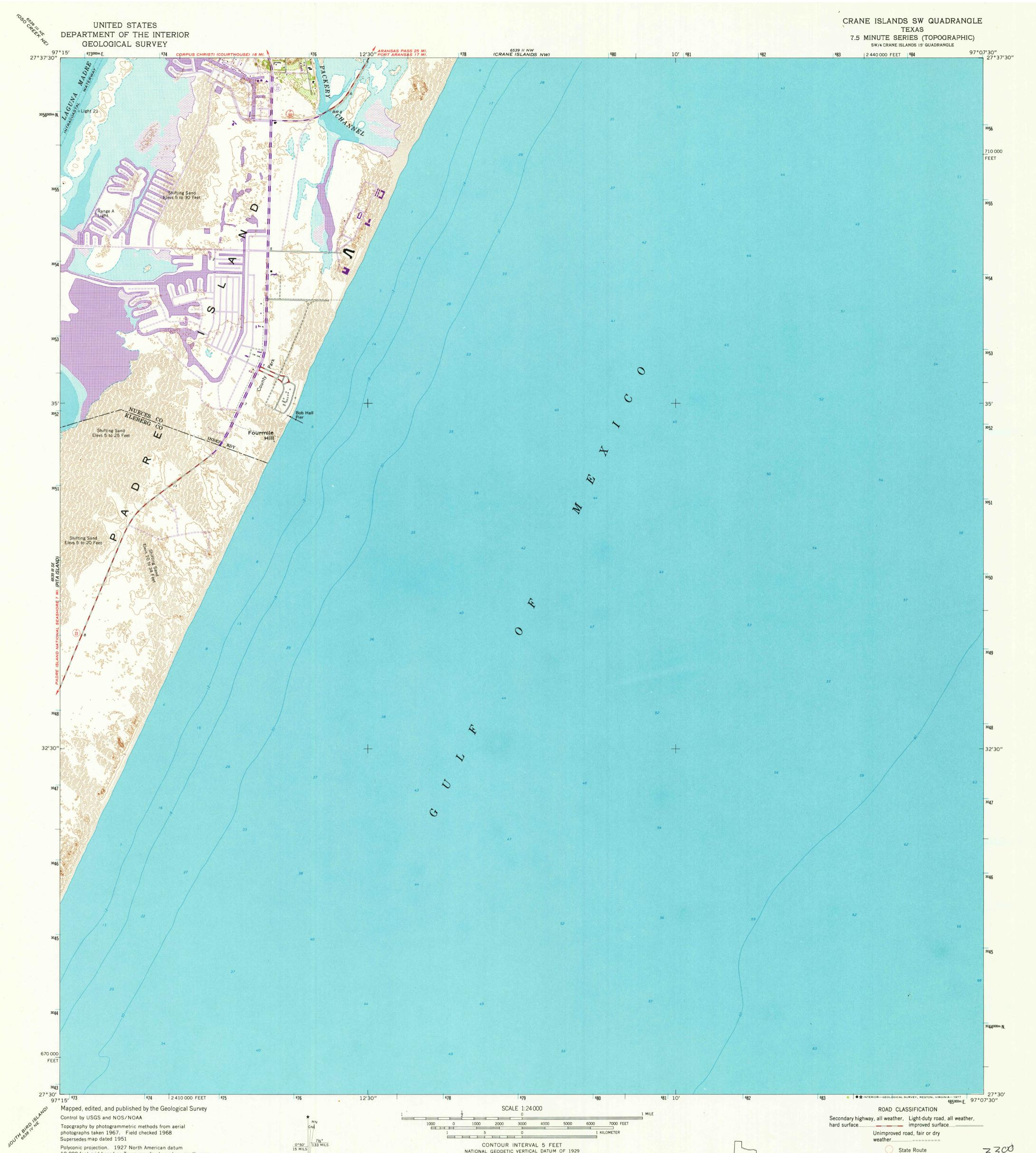
Polyconic projection. 1927 North American datum 10,000-foot grid based on Texas coordinate system, south zone 1000-meter Universal Transverse Mercator grid ticks, zone 14, shown in blue
