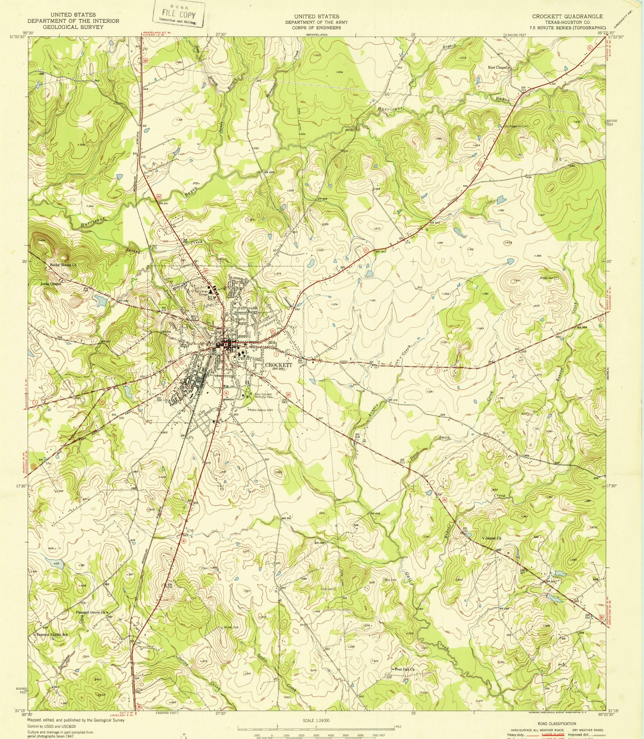
Topography by plane-table methods 1949-1950 Polyconic projection. 1927 North American datum 10,000-foot grid based on Texas coordinate system, central zone
