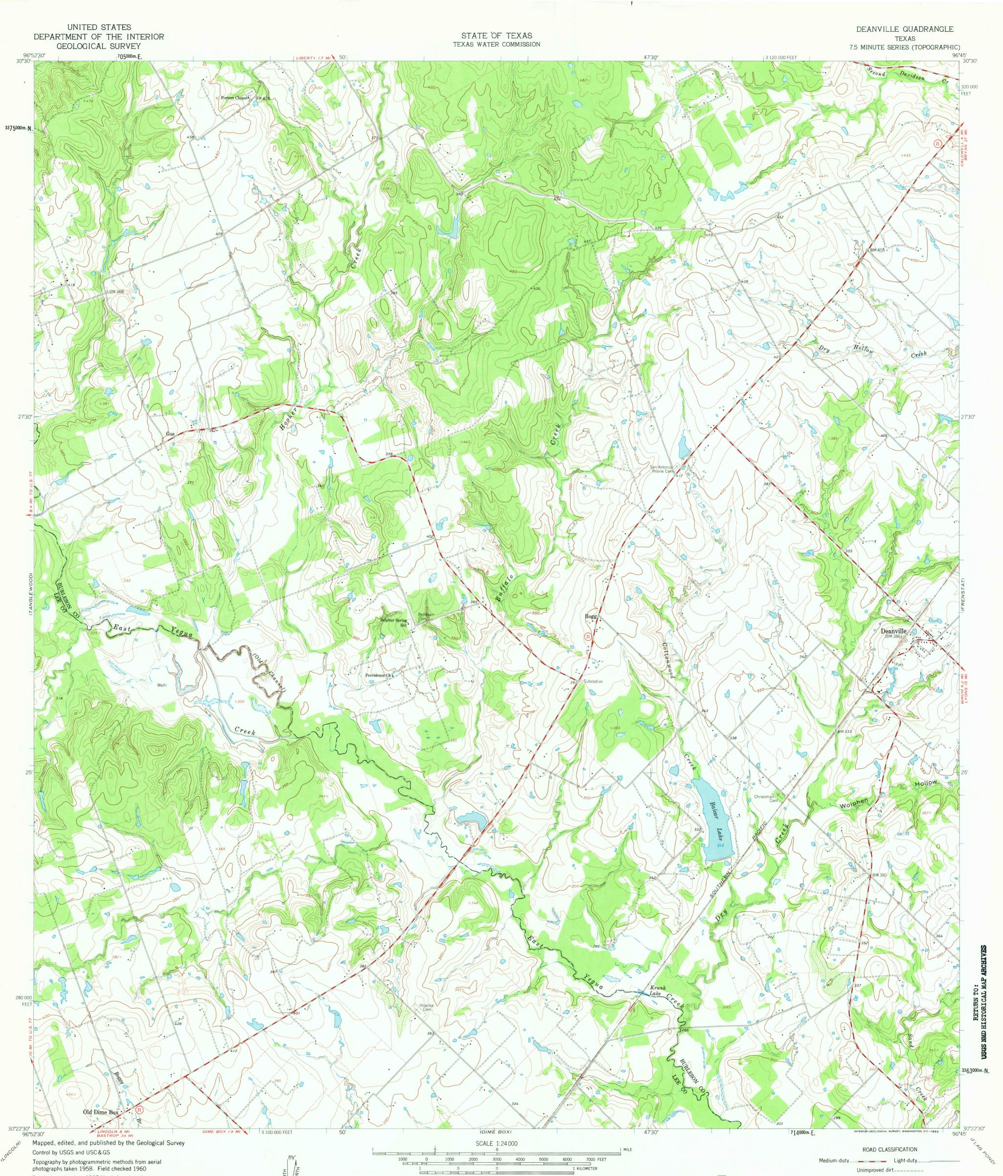
Polyconic projection. 1927 North American datum 10,000-foot grid based on Texas coordinate system, central zone 1000-meter Universal Transverse Mercator grid ticks, zone 14, shown in blue Fine red dashed lines indicate selected fence and field lines where
