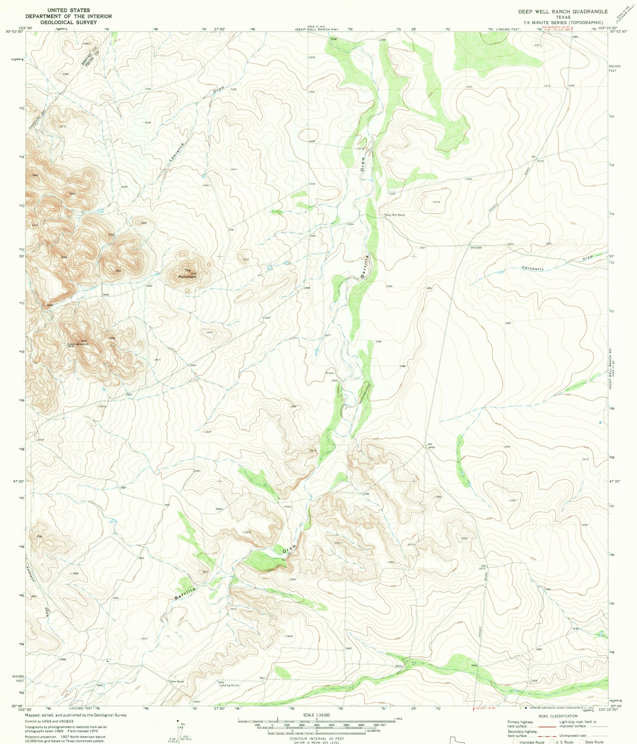
10,000-foot grid based on Texas coordinate system, central zone 1000-meter Universal Transverse Mercator grid ticks, zone 13, shown in blue
