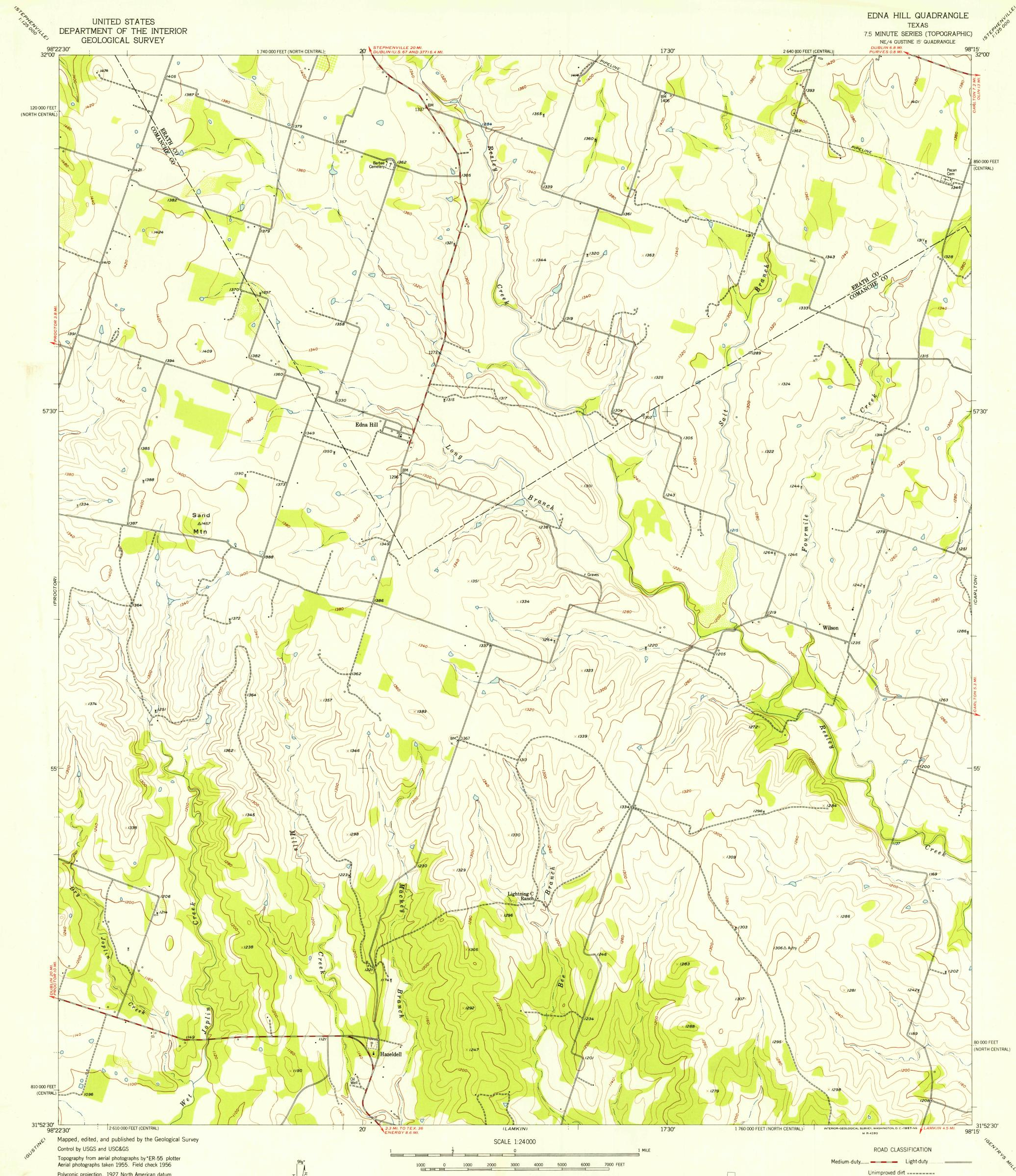
Polyconic projection. 1927 North American datum 10,000-foot grid based on Texas coordinate system, central and north central zones
