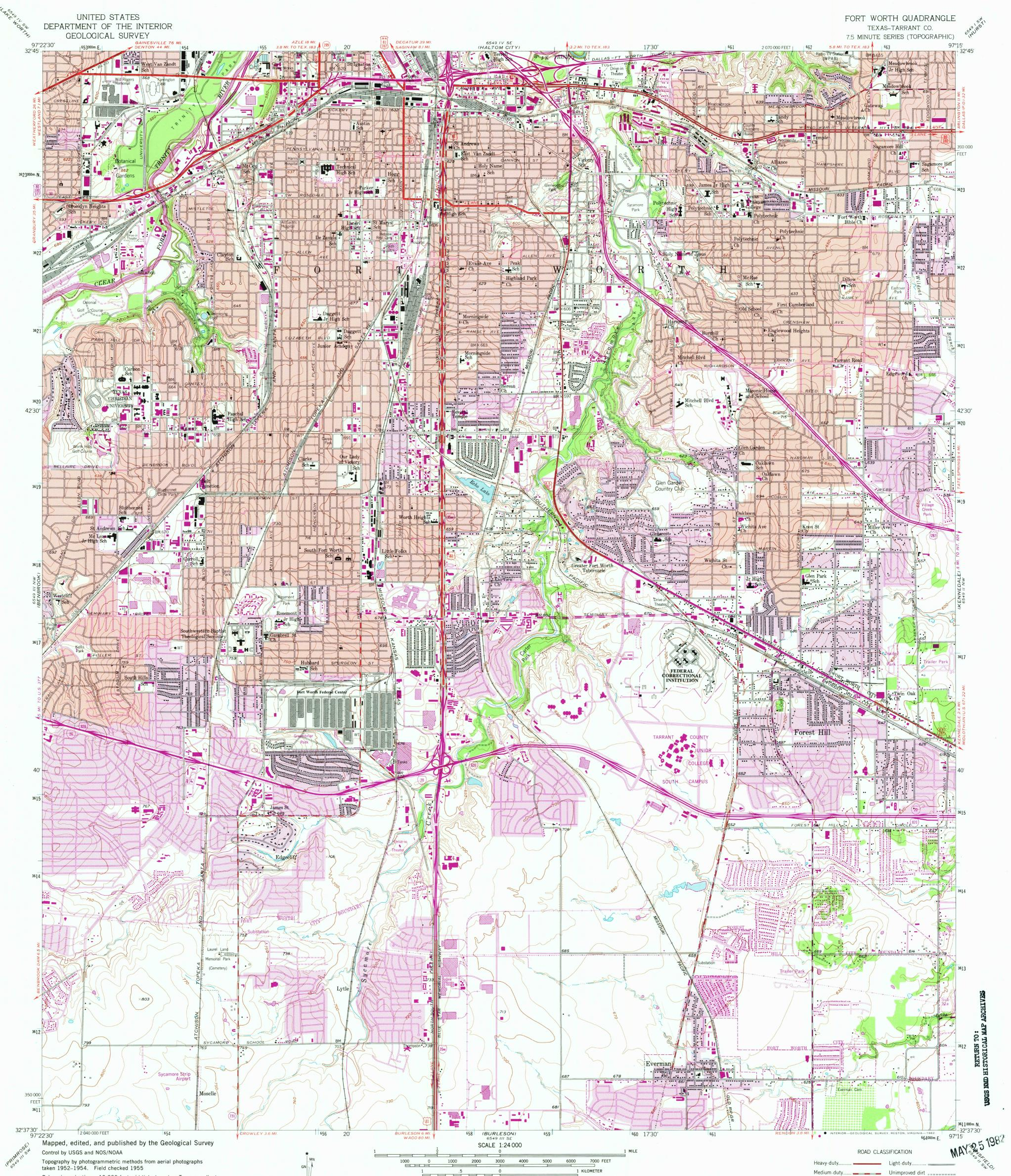
Polyconic projection. 10,000-foot grid ticks based on Texas coordinate system, north central zone. 1000-meter Universal Transverse Mercator grid ticks, zone 14, shown in blue. 1927 North American Datum To place on the predicted North American Datum 1983 move the projection lines 10 meters south and 28 meters east as shown by dashed corner ticks
