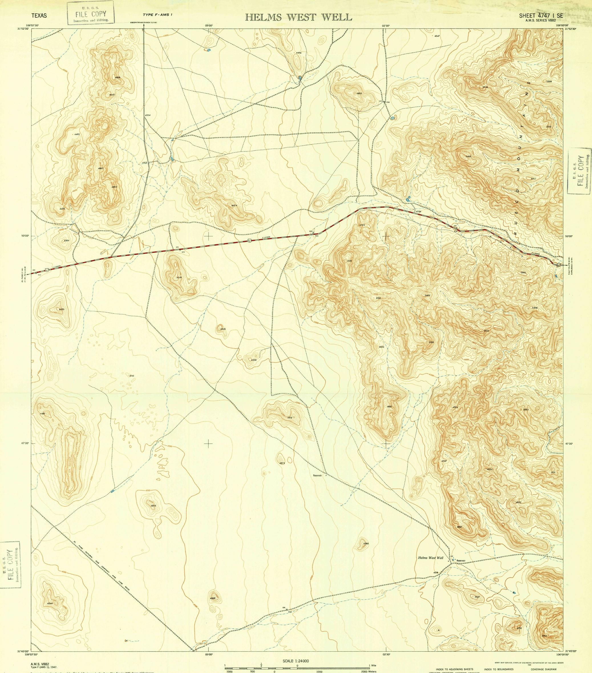
Prepared under the direction of the Chief of Engineers by the Army Map Service (AM), Corps of Engineers, Department of the Army, Washington, D. C. Compiled in 1947 from Texas, 1:62,500, USGS, Hueco Tanks, 1944. Planimetric detail revised from aerial photography by photo-planimetric methods. Aerial photography by U. S. Air Force, 1944-46. Horizontal and vertical control by USC&GS. Planimetry field edited 1947.
