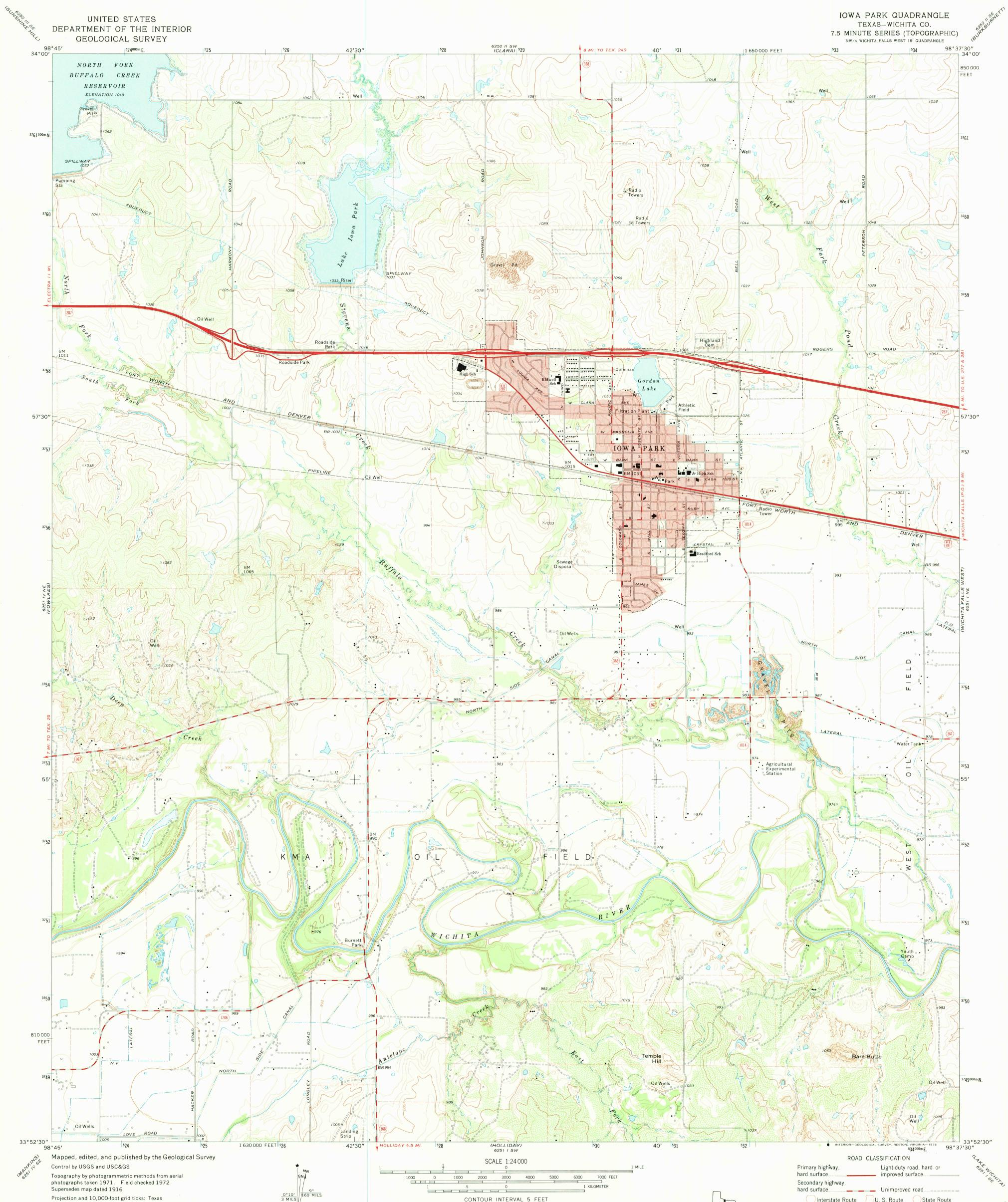
Projection and 10,000-foot grid ticks: Texas coordinate system, north central zone (Lambert conformal conic) 1000-meter Universal Transverse Mercator grid ticks, zone 14, shown in blue. 1927 North American datum Red tint indicates areas in which only landmark buildings are shown Fine red dashed lines indicate selected fence lines
