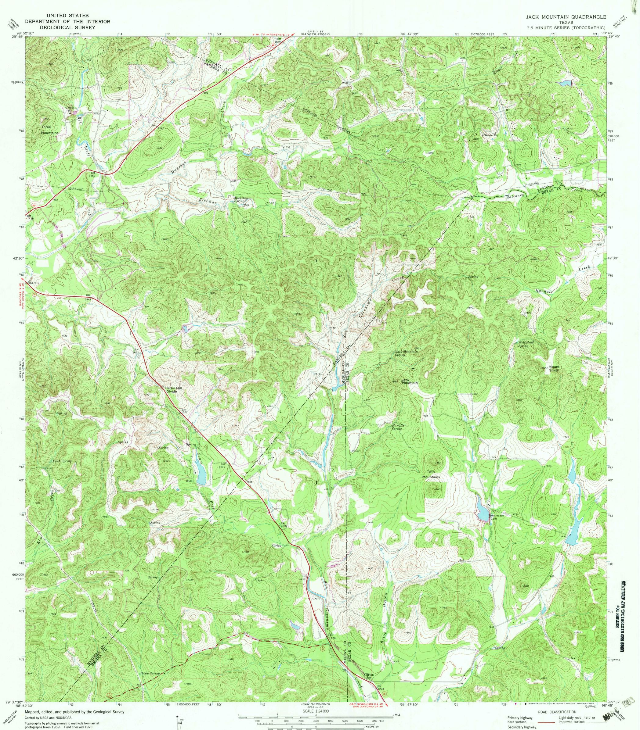
Polyconic projection. 10,000-foot grid ticks based on Texas coordinate system, south central zone. 1000-meter Universal Transverse Mercator grid ticks, zone 14, shown in blue. 1927 North American Datum. To place on the predicted North American Datum 1983 move the projection lines 20 meters south and 30 meters east as shown by dashed corner ticks Fine red dashed lines indicate selected fence lines
