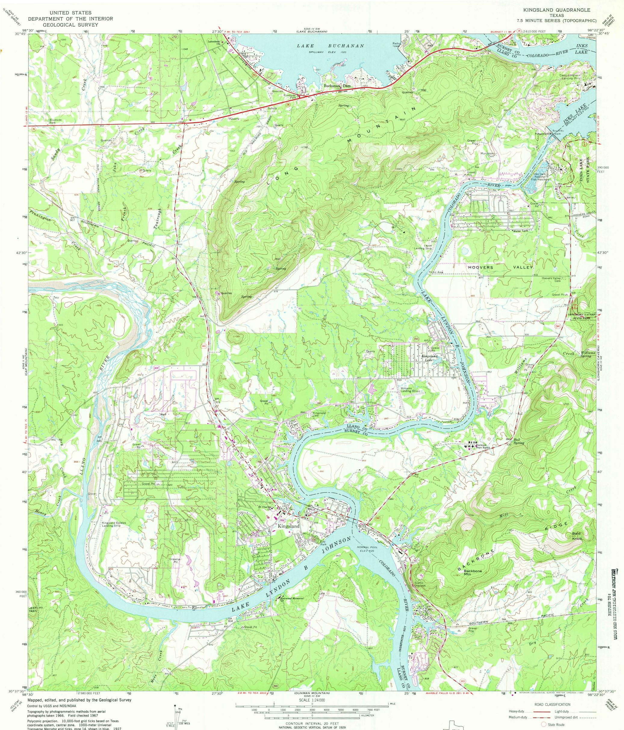
coordinate system, central zone. 1000-meter Universal Transverse Mercator grid ticks, zone 14, shown in blue. 1927 North American Datum. To place on the predicted North American Datum 1983 move the projection lines 16 meters south and 30 meters east as shown by dashed corner ticks Fine red dashed lines indicate selected fence lines
