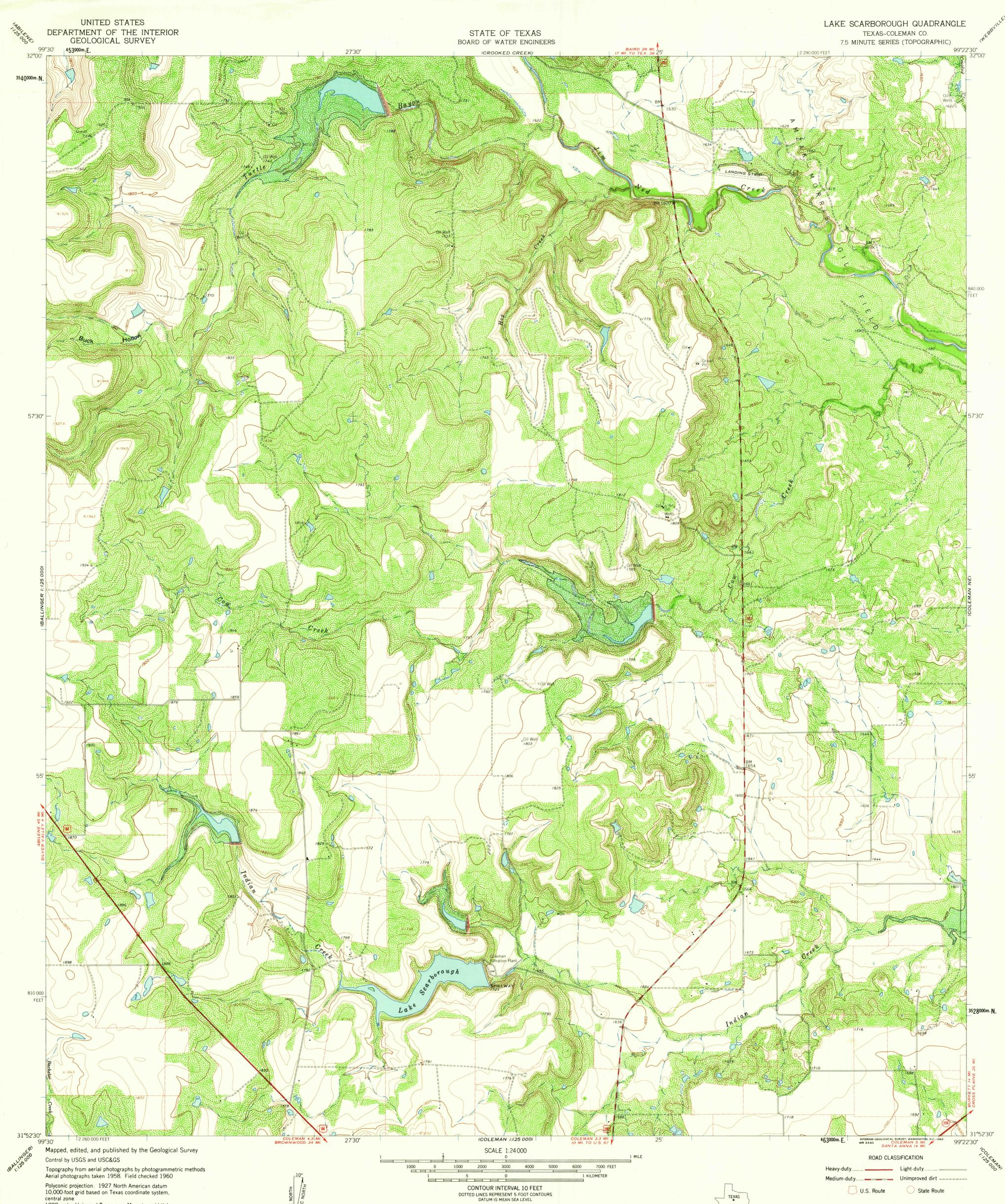
Polyconic projection. 1927 North American datum 10,000-foot grid based on Texas coordinate system, central zone 1000-meter Universal Transverse Mercator grid ticks, zone 14, shown in blue
