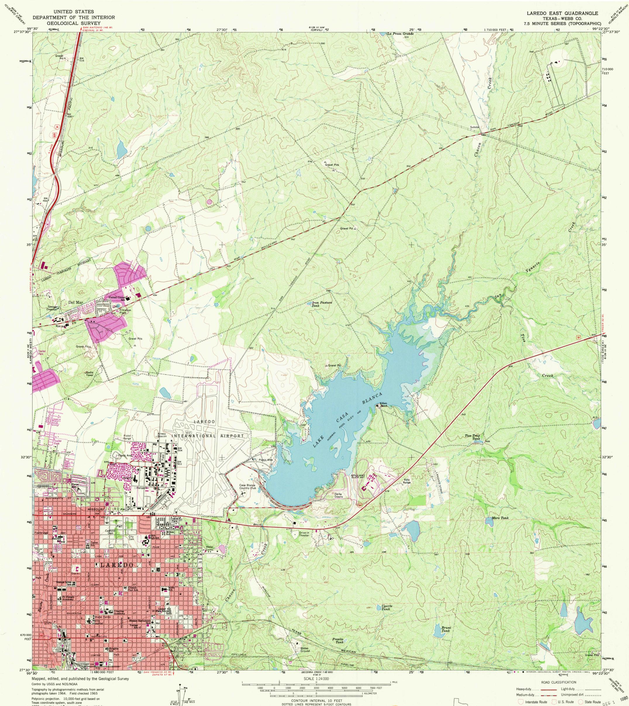
Texas coordinate system, south zone 1000-meter Universal Transverse Mercator grid ticks, zone 14, shown in blue. 1927 North American Datum To place on the predicted North American Datum 1983 move the projection lines 27 meters south and 32 meters east as shown by dashed corner ticks Red tint indicates area in which only landmark buildings are shown Fine red dashed lines indicate selected fence lines
