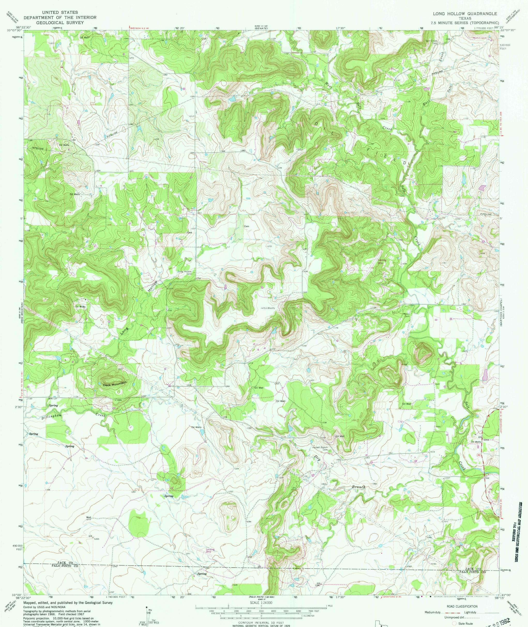
Polyconic projection. 10,000-foot grid ticks based on Texas coordinate system, north central zone. 1000-meter Universal Transverse Mercator grid ticks, zone 14, shown in blue. 1927 North American Datum. To place on the predicted North American Datum 1983 move the projection lines 9 meters south and 31 meters east as shown by dashed corner ticks
