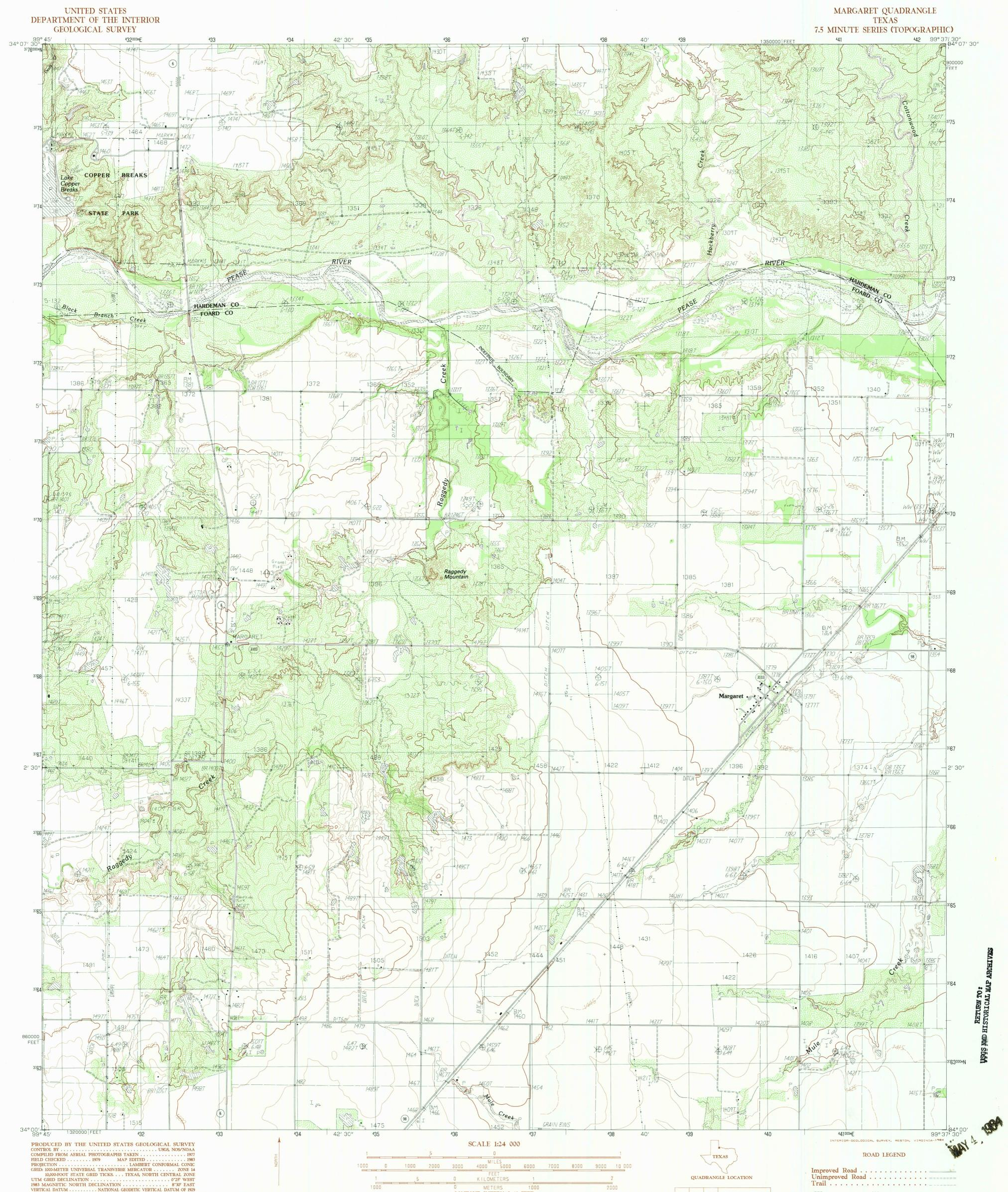
VERTICAL DATUM ...... NATIONAL GEODETIC VERTICAL DATUM OF 1929 HORIZONTAL DATUM ...... 1927 NORTH AMERICAN DATUM To place on the predicted North American Datum of 1983, move the projection lines as shown by dashed corner ticks (4 meters south and 35 meters east) There may be private inholdings within the boundaries of any Federal and State Reservations shown on this map All marginal data and lettering generated and positioned by automated type placement procedures
