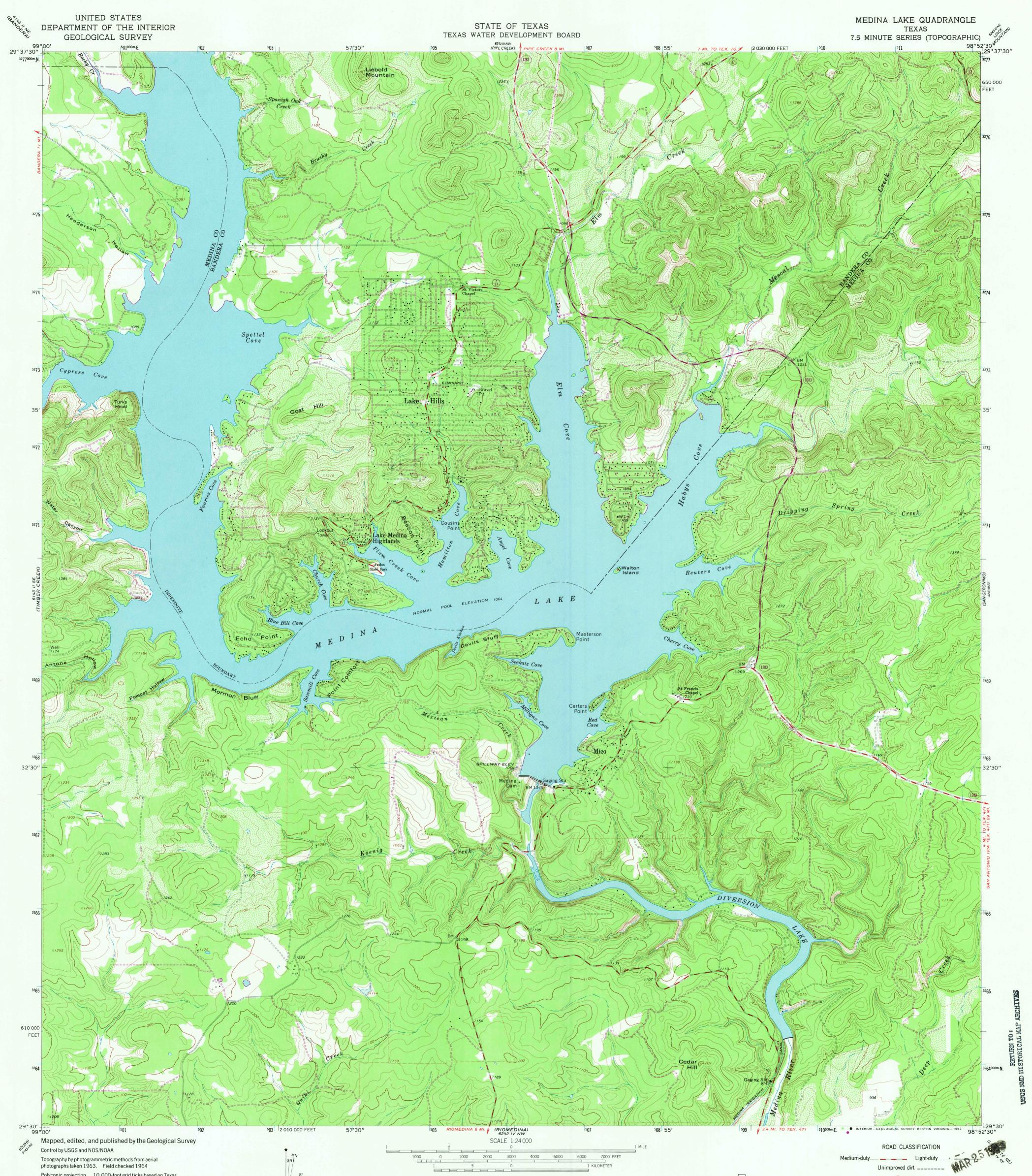
Polyconic projection. 10,000-foot grid ticks based on Texas coordinate system, south central zone. 1000-meter Universal Transverse Mercator grid ticks, zone 14, shown in blue. 1927 North American Datum. To place on the predicted North American Datum 1983 move the projection lines 20 meters south and 30 meters east as shown by dashed corner ticks
