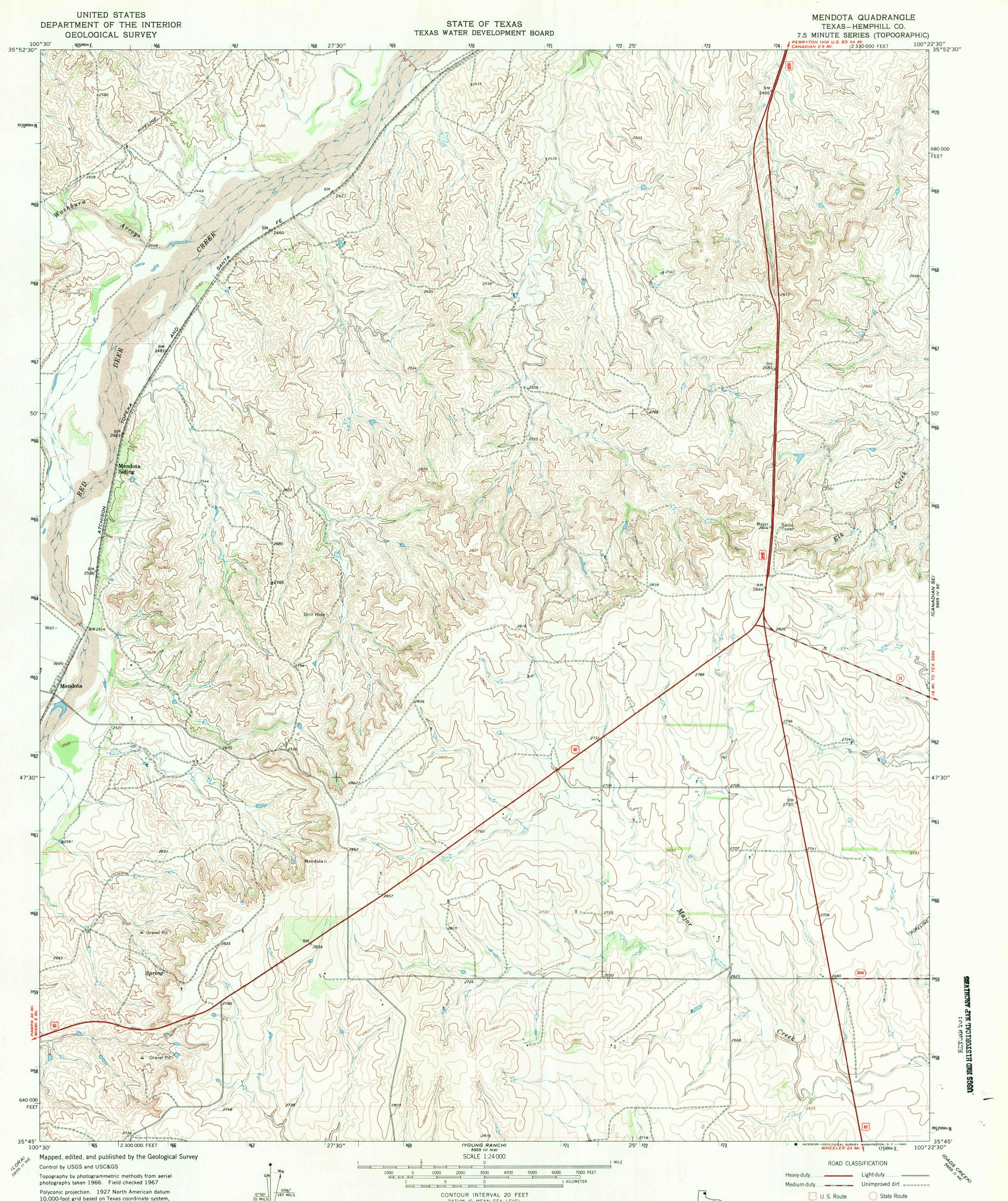
10,000-foot grid based on Texas coordinate system, north zone 1000-meter Universal Transverse Mercator grid ticks, zone 14, shown in blue
