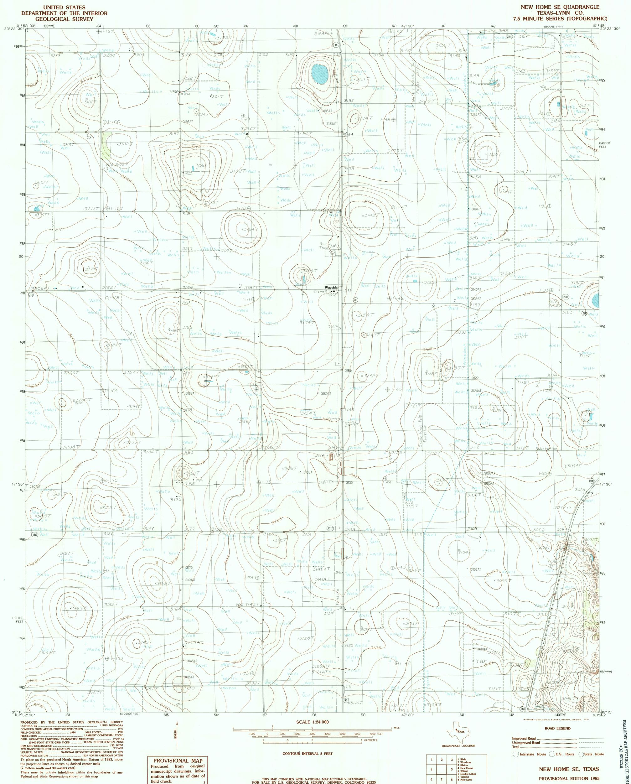
1985 MAGNETIC NORTH DECLINATION ..... 9° EAST ..... NATIONAL GEODETIC VERTICAL DATUM OF 1929 VERTICAL DATUM ..... ........ 1927 NORTH AMERICAN DATUM HORIZONTAL DATUM ..... To place on the predicted North American Datum of 1983, move the projection lines as shown by dashed corner ticks (7 meters south and 30 meters east) There may be private inholdings within the boundaries of any Federal and State Reservations shown on this map
