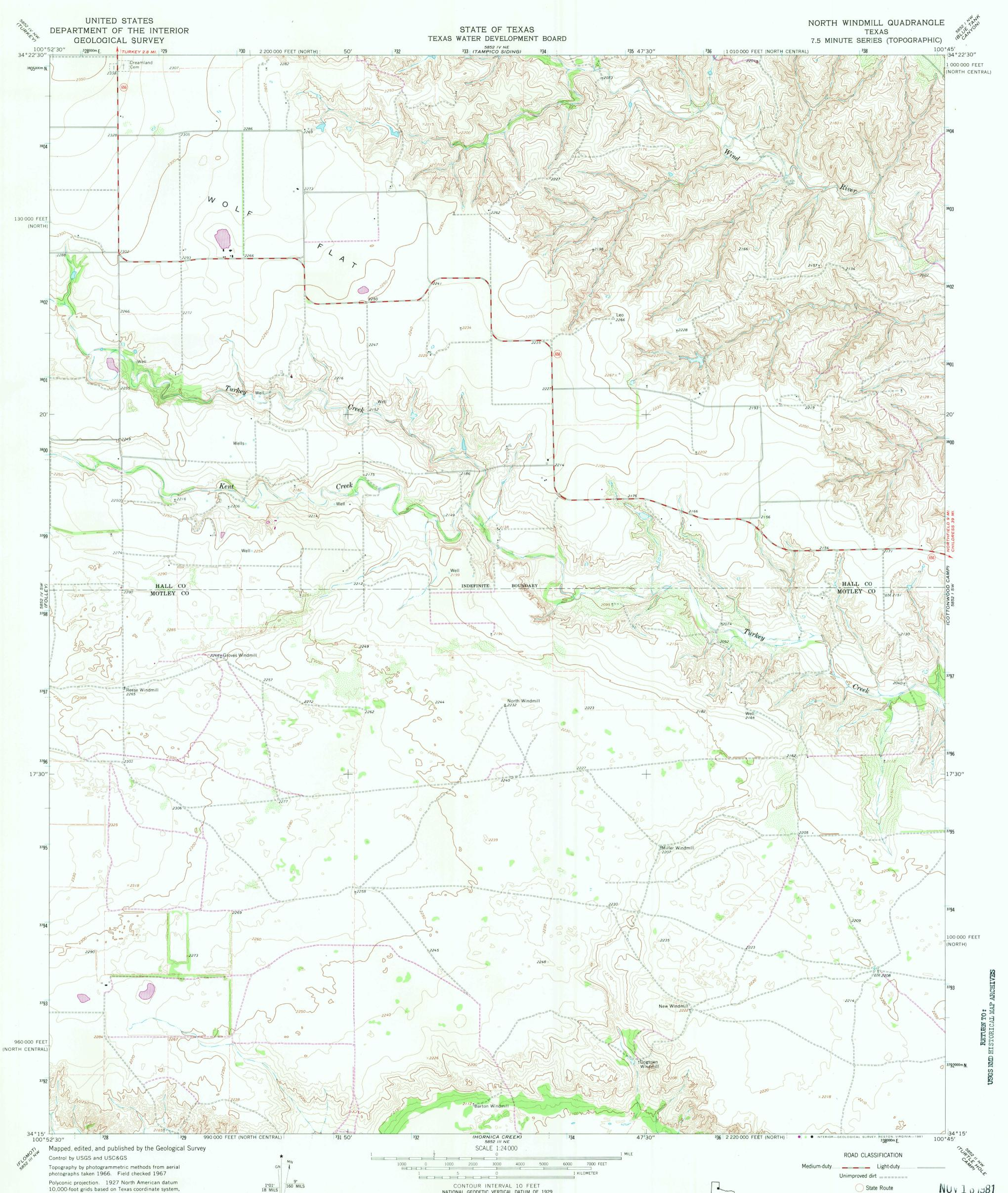
Polyconic projection. 1927 North American datum 10,000-foot grids based on Texas coordinate system, north central and north zones 1000-meter Universal Transverse Mercator grid ticks, zone 14, shown in blue
