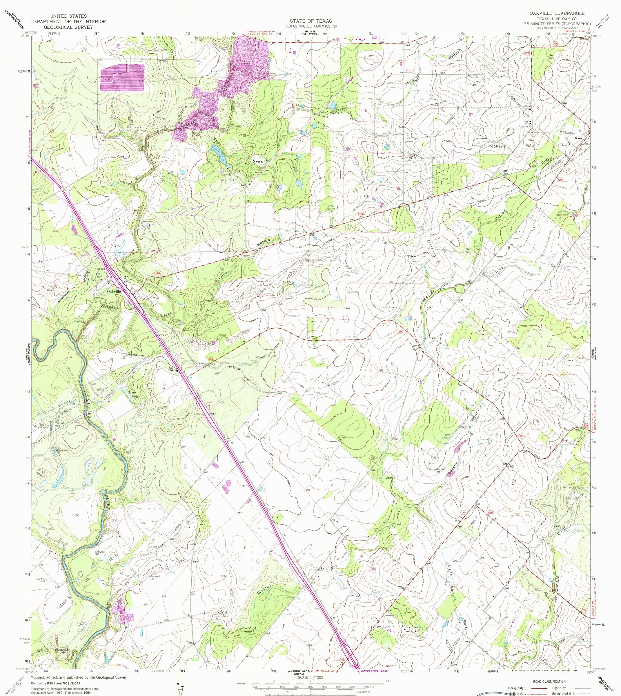
Polyconic projection. **1927 North American Datum** 10,000-foot grid based on Texas coordinate system, south central zone 1000-meter Universal Transverse Mercator grid ticks, zone 14, shown in blue
