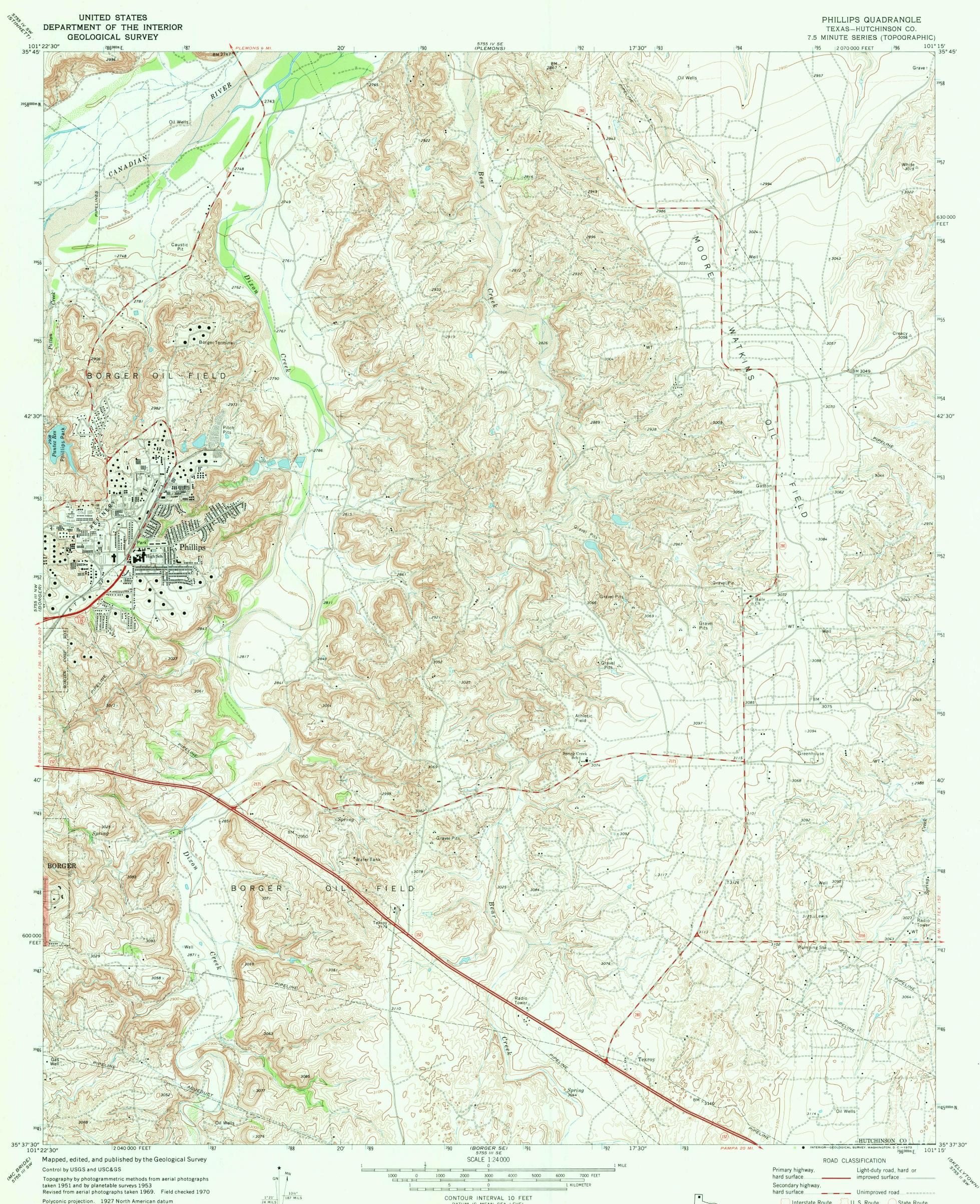
Polyconic projection. 1927 North American datum 10,000-foot grid based on Texas coordinate system, north zone 1000-meter Universal Transverse Mercator grid ticks, zone 14, shown in blue Red tint indicates areas in which only landmark buildings are shown
